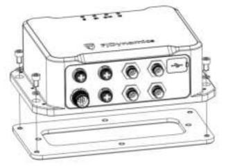
The machine control box is fixed to the control box fixed base with 4 screws and 4 standard spring washers, as shown in the above figure. The control box fixed base can be welded and fixed in the appropriate position of the excavator, or four magnets can be installed (as shown in the figure below, magnets fixed to the base with screws) and then attached to the appropriate position of the excavator.
