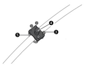
Fix the bracket base. Select an appropriate position inside the cab for easy operation. Then, fix the control terminal bracket base there with U-bolts and nuts .
