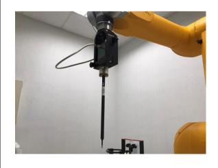
Probe setup on robot
