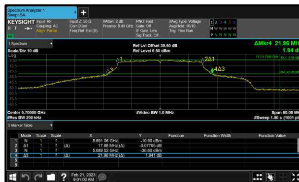
Figure 264 - 802.11ac HT20 Maximum 99% OBW
