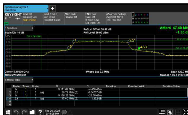
Figure 266 - 802.11ac HT40 Maximum 99% OBW
