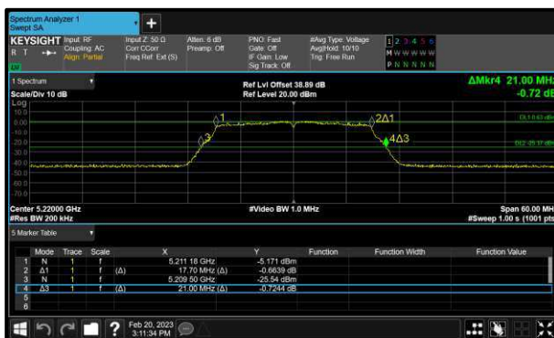
Figure 263 - 802.11ac HT20 Minimum 99% OBW
