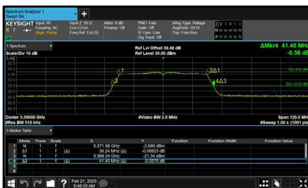
Figure 265 - 802.11ac HT40 Minimum 99% OBW
