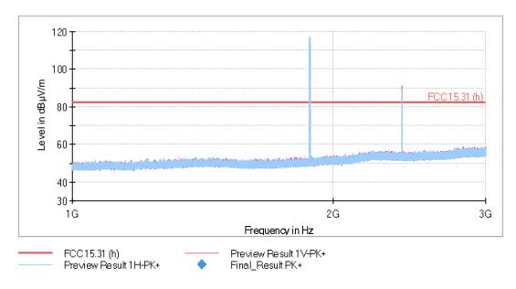
The peak on the left above the limit is the 2G 1900 carrier frequency. The peaks on the right above the limit are the BLE carrier frequency.
