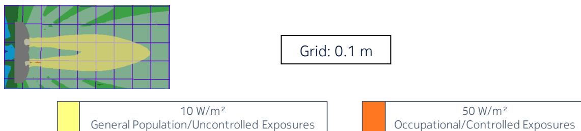
Figure 4 – Top view of the power density for the time-averaged actual maximum transmitted power of 0.178 W and the beam oriented in azimuth = 0° & elevation = 0°
