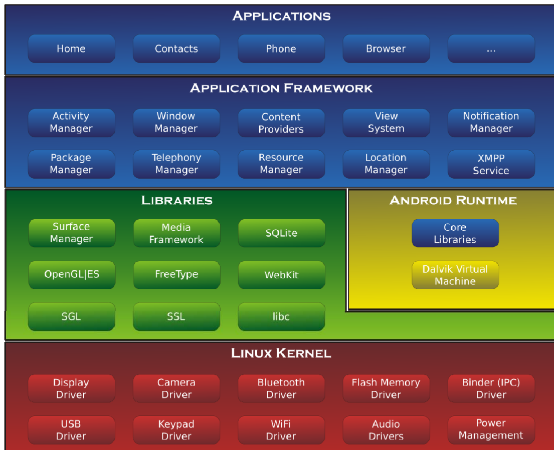
Fig 2-1. Android System Structure
