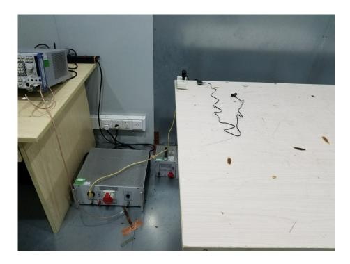
Radiation Emission Test Setup (Below 30MHz)
