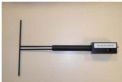
Figure 1 – Satimo COMOSAR Validation Dipole
