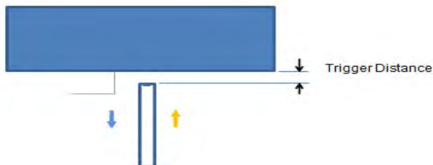
Picture: Proximity sensor triggering distances assessment (Bottomside)
