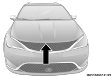
Safety Latch Release Lever Location
