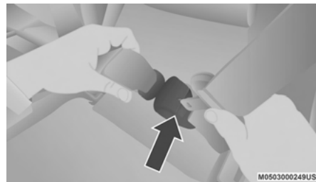
Detaching Mini-Buckle With Seat Belt Tongue
