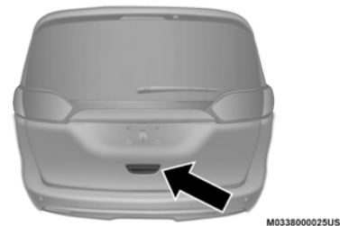
Unlock Liftgate Using Passive Entry
