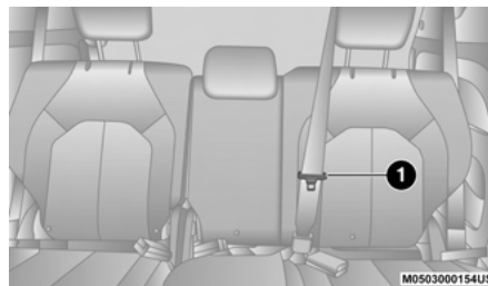
Routing The Rear Seat Belt Latch Plate
