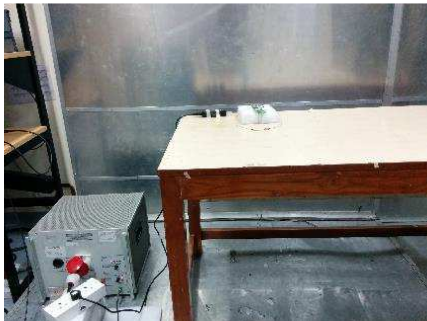
Figure 14: Conducted Emission Test set up photograph – 150 kHz to 30 MHz
