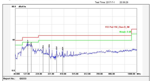
Test Standard: FCC Part 15C\_Class B\_3M
