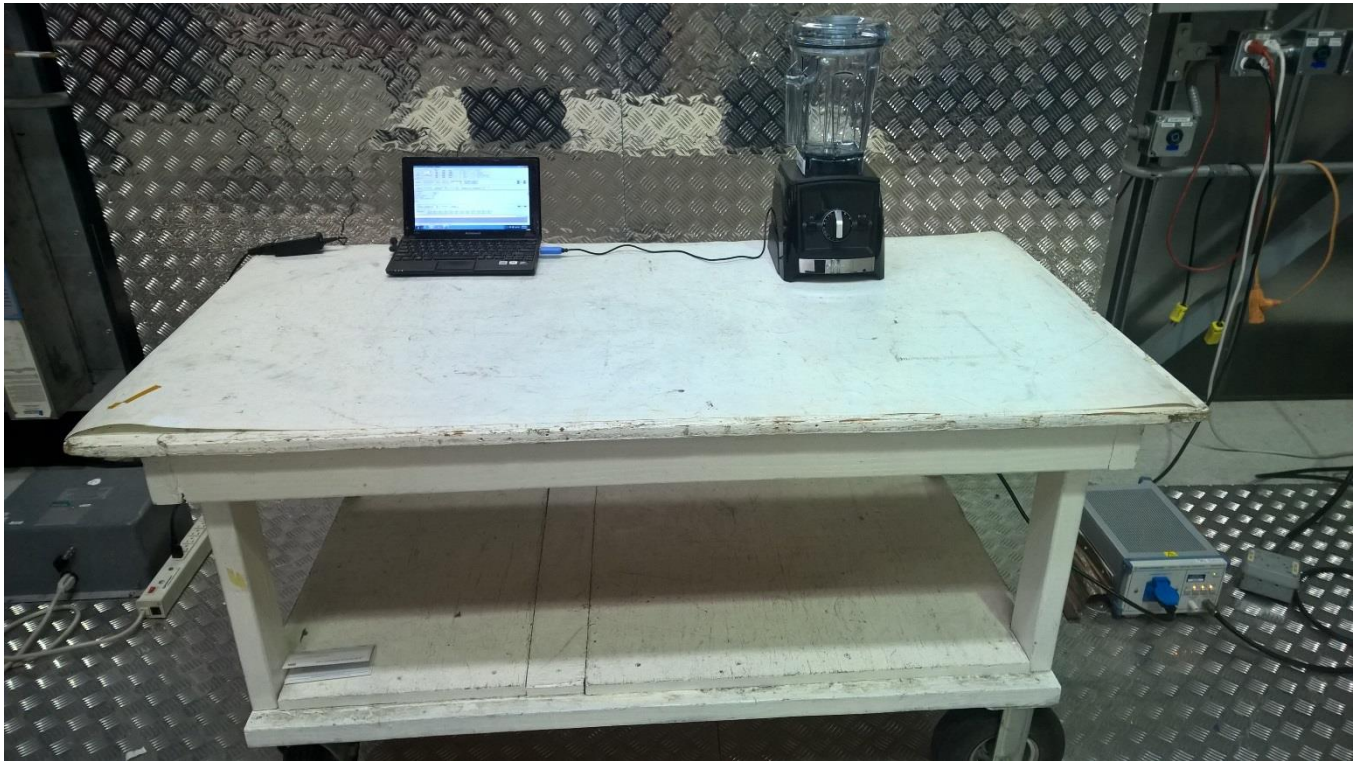
Figure 3.6-3: AC Powerline Conducted Emissions Setup
