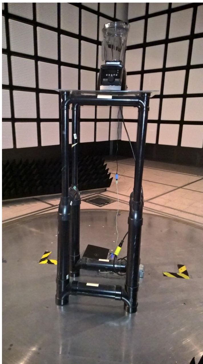
Figure 3.6-2: Radiated Emissions Test Setup – above 1GHz
