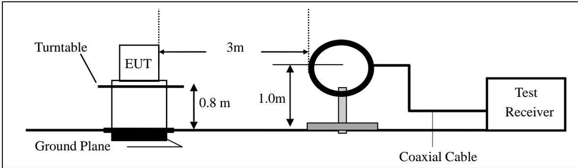
(b) For radiated emissions from 30MHz to 1000MHz
