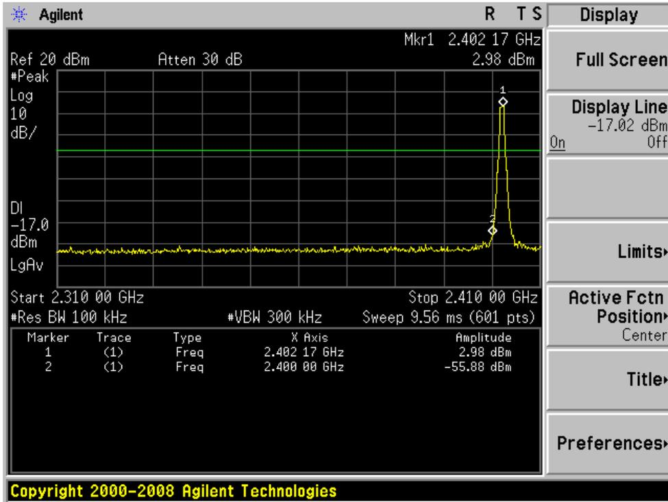
GFSK mode: Band Edge-High Channel
