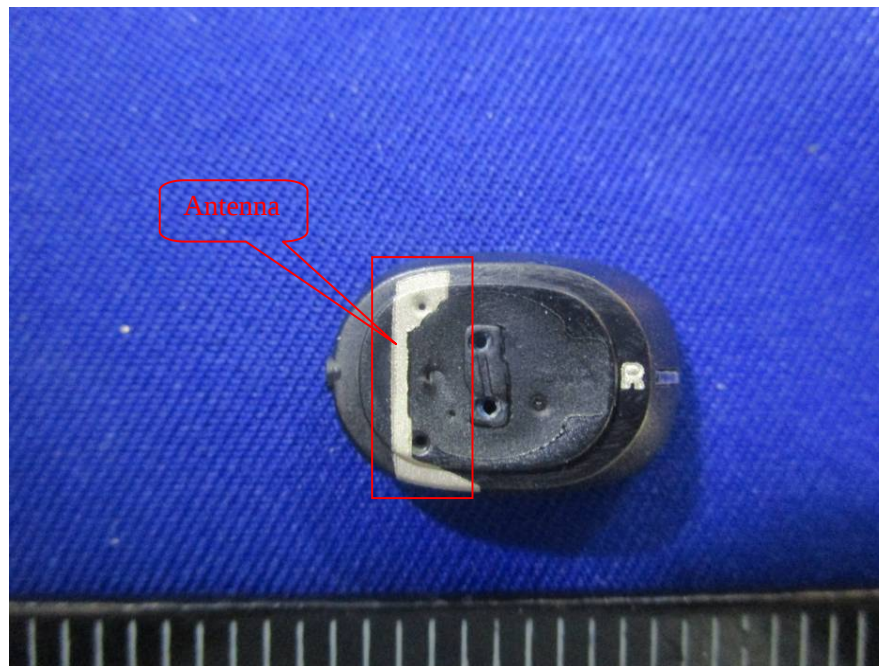
EUT – Right Earbud Antenna View
