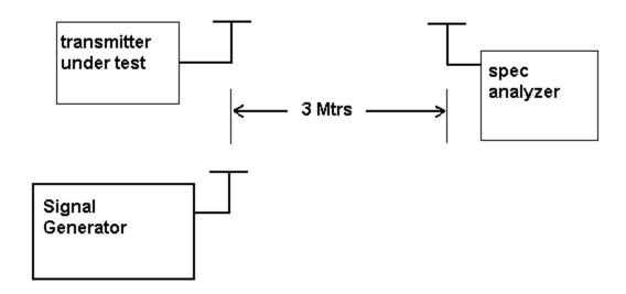
Equipment placed 80 cm above ground on a rotatable platform.
