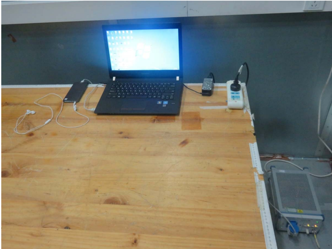
Picture 2 Conducted Emission Test Setup
