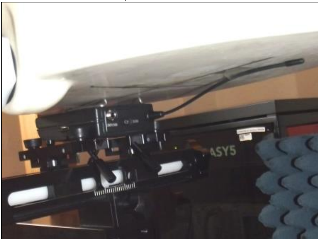
Photo 6: Test position - Rear with 0mm distance
