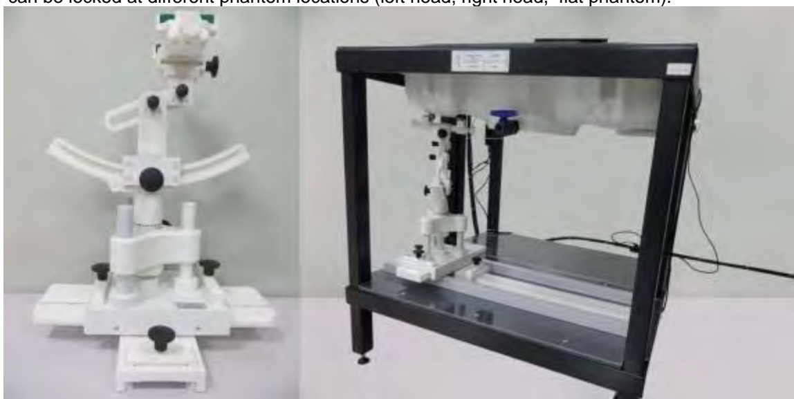
Device holder supplied by SATIMO
