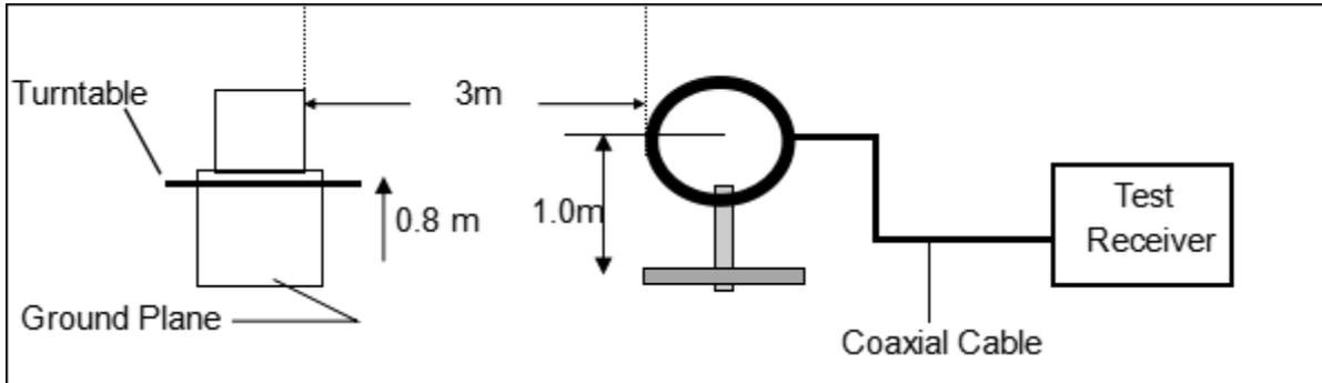
(b) For Radiated Emission 30~1000MHz
