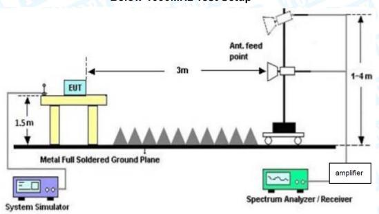
**Above 1GHz Test Setup**
