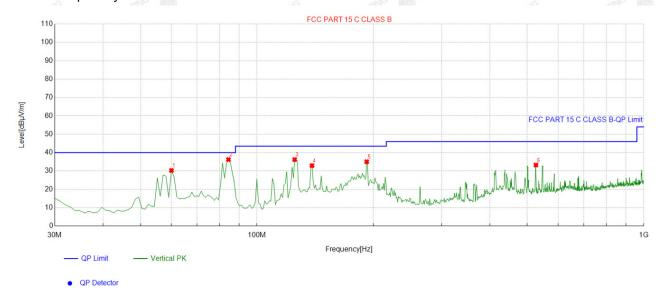
Suspected List Freq. Factor Reading Level Limit Margin Height Angle NO. **Polarity** [dB] [MHz]  $[dB\mu V/m]$  $[dB\mu V/m]$  $[dB\mu V/m]$ [dB] [cm] 60.1001 -14.37 44.63 40.00 30.26 9.74 100 346 Vertical 2 84.374374 -17.86 54.04 36.18 40.00 3.82 100 330 Vertical 52.30 43.50 100 358 Vertical 125.15515 -16.11 36.19 7.31 4 138.74874 100 Vertical -17.81 50.73 32.92 43.50 10.58 330 5 51.78 192.15215 -16.74 35.04 43.50 8.46 100 359 Vertical 6 526.16616 -7.06 40.28 33.22 46.00 12.78 100 359 Vertical
