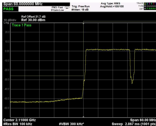
Low Band Edge, 2 Carrier, Modulation: 64QAM, BW=20MHz
