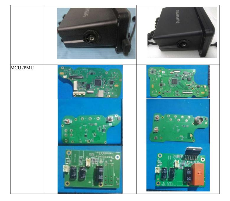
Note: For the appearance, the differences are the size (RF main board, PCB layout and RF characteristics are the same.) and the Front keypad and backend interface.
