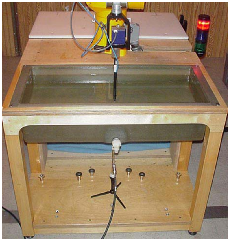
DASY4 SAR Measurement System with planar phantom
