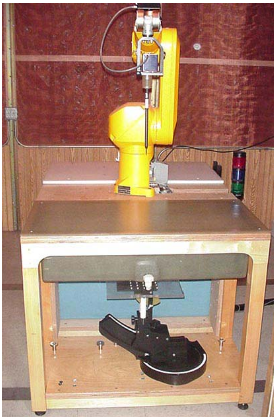
DASY4 SAR Measurement System with planar phantom
