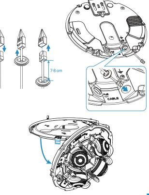
**Note:** The grommet should be pulled from the outside to the inside to ensure its waterproof and airtight properties.
