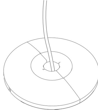
5. Pass the power cord through the hole of the screw nut and tighten the screw with the base plate.
