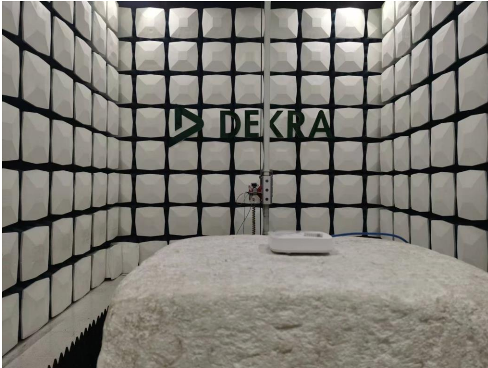
Description: Radiated Emission Test Setup for 1~18GHz
