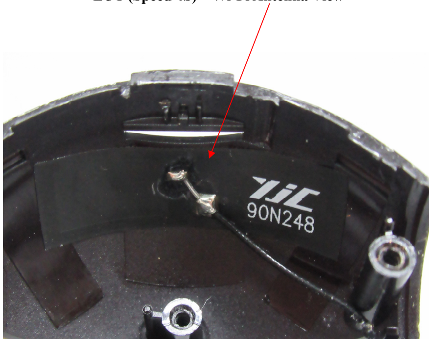
EUT (Speed 4S) – Wi-Fi Antenna View
