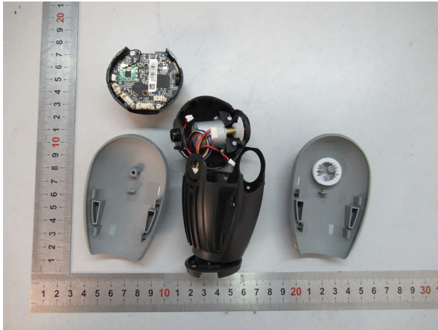
EUT (Speed 4S) – Cover off View-2
