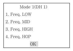
f. Selecting "Freq. LOW" item will transmit DH 1 packet in low cannel. You can see screen below. You will select [OK] soft key to exit this menu.
