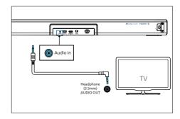
Use a RCA to 3.5mm audio cable to connect the TV's audio output sockets to the AUX socket on the unit.
