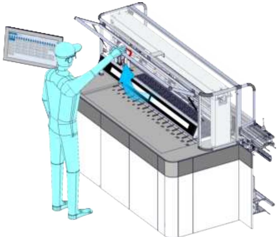
5. Grasp the robot and manually slide it on the side of the Module to allow easy access to the area.
