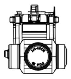
PTZ of EVO Nano+ Support 4K camera with 1/1.28 inch CMOS sensor
