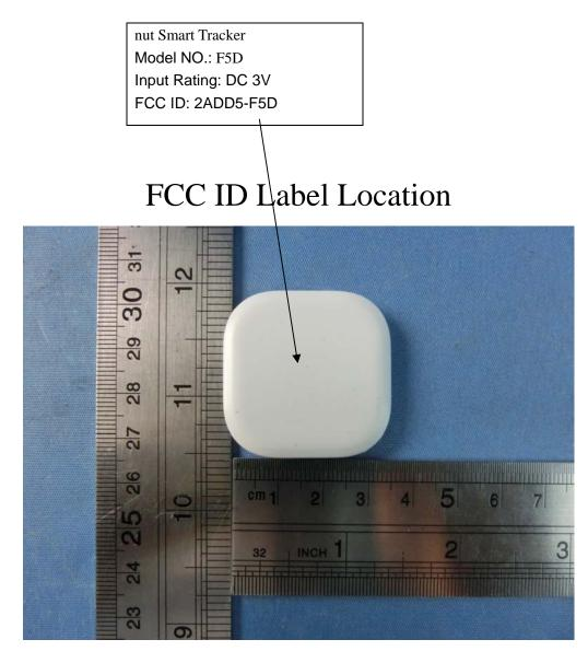
The label shown shall be permanently affixed at a conspicuous location on the device and be readily visible to the user at the time purchase (Labeling requirements per 2.925)
