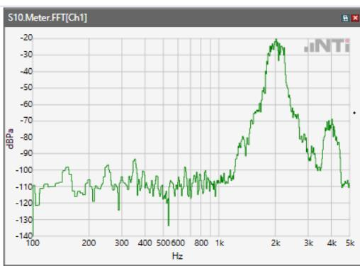
ANSI/TIA 5050-2018 \ 2N HAC ON \ NB 12.2kbps\ 5.2 Receive path – distortion and noise\LTE Band 66
