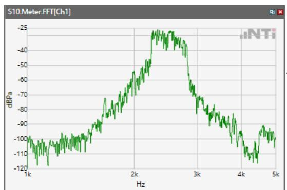
ANSI/TIA 5050-2018 \ 2N HAC ON \ NB 12.2kbps\ 5.2 Receive path – distortion and noise\LTE Band 66
