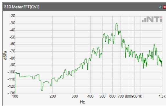
ANSI/TIA 5050-2018 \ 8N HAC OFF \ WB 23.85 kbps\ 5.2 Receive path – distortion and noise\LTE Band 2
