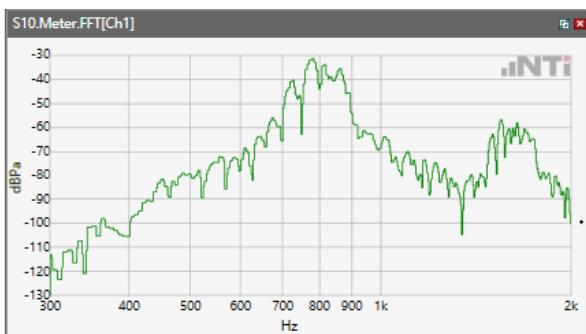
ANSI/TIA 5050-2018 \ 2N HAC ON \ NB 12.2kbps\ 5.2 Receive path – distortion and noise\WCDMA Band IV
