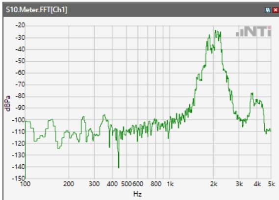
ANSI/TIA 5050-2018 \ 8N HAC OFF \ WB 23.85 kbps\ 5.2 Receive path – distortion and noise\GSM 1900
