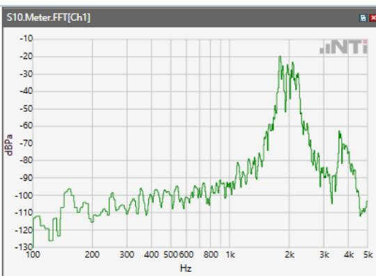
ANSI/TIA 5050-2018 \ 2N HAC ON \ NB 12.2kbps\ 5.2 Receive path – distortion and noise\LTE BAND 71
