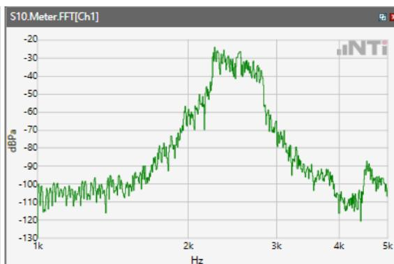
ANSI/TIA 5050-2018 \ 8N HAC OFF \ NB 12.2kbps\ 5.2 Receive path – distortion and noise\WCDMA Band IV
