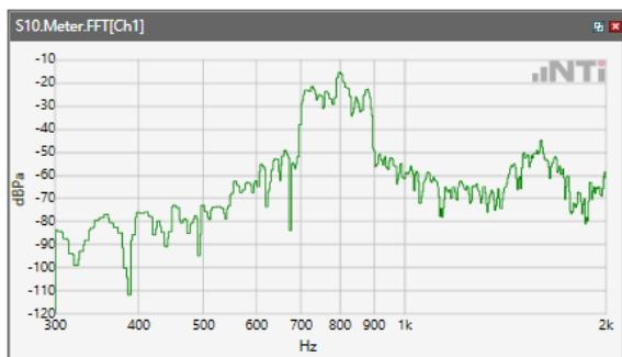
ANSI/TIA 5050-2018 \ 2N HAC ON \ NB 12.2kbps\ 5.2 Receive path – distortion and noise\LTE Band 5
