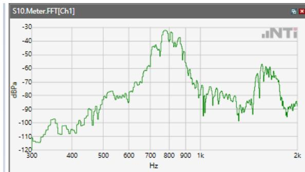
ANSI/TIA 5050-2018 \ 2N HAC ON \ NB 12.2kbps\ 5.2 Receive path – distortion and noise\GSM 1900
