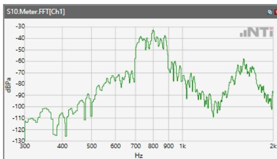
ANSI/TIA 5050-2018 \ 8N HAC OFF \ WB 23.85 kbps\ 5.2 Receive path – distortion and noise\WCDMA IV
