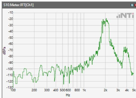
ANSI/TIA 5050-2018 \ 8N HAC OFF \ NB 12.2kbps\ 5.2 Receive path – distortion and noise\LTE Band 66
