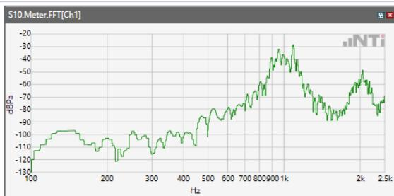
ANSI/TIA 5050-2018 \ 2N HAC ON \ NB 12.2kbps\ 5.2 Receive path – distortion and noise\GSM 1900
