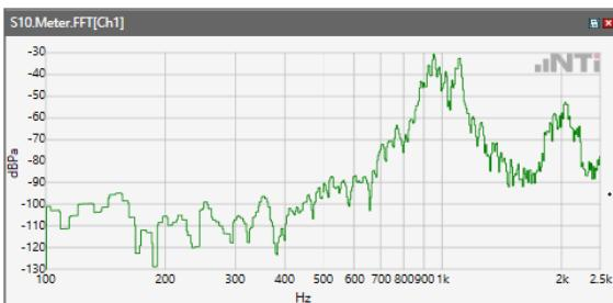
ANSI/TIA 5050-2018 \ 8N HAC OFF \ NB 12.2kbps\ 5.2 Receive path – distortion and noise\WCDMA Band V
