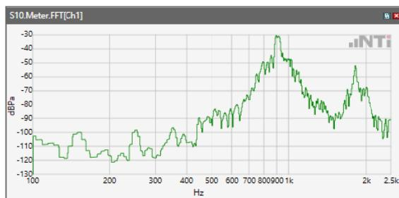
ANSI/TIA 5050-2018 \ 8N HAC OFF \ NB 12.2kbps\ 5.2 Receive path – distortion and noise\LTE Band 2
