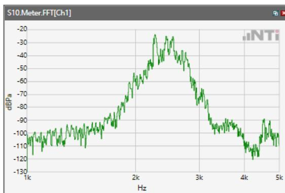
ANSI/TIA 5050-2018 \ 2N HAC ON \ NB 12.2kbps\ 5.2 Receive path – distortion and noise\LTE BAND 71
