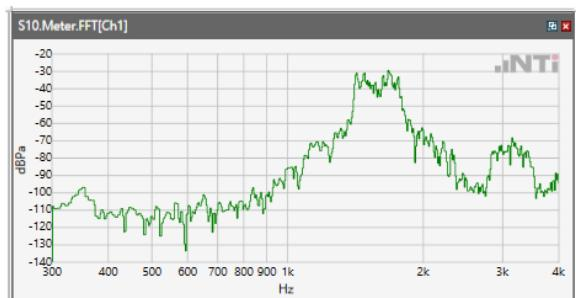
ANSI/TIA 5050-2018 \ 2N HAC ON \ NB 12.2kbps\ 5.2 Receive path – distortion and noise\LTE Band 66
