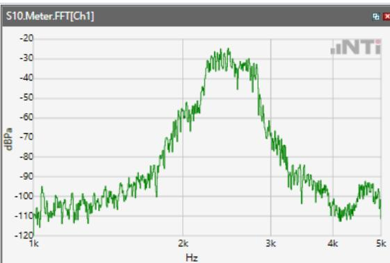
ANSI/TIA 5050-2018 \ 8N HAC OFF \ NB 12.2kbps\ 5.2 Receive path – distortion and noise\WCDMA Band II
