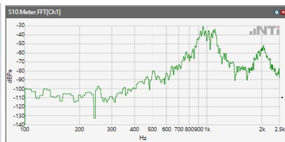
ANSI/TIA 5050-2018 \ 2N HAC ON \ NB 12.2kbps\ 5.2 Receive path – distortion and noise\WCDMA Band II
