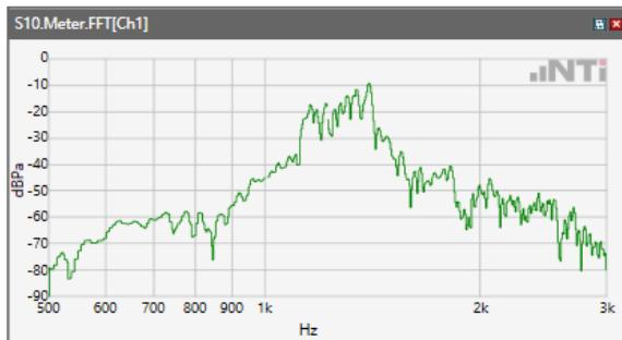
ANSI/TIA 5050-2018 \ 2N HAC ON \ NB 12.2kbps\ 5.2 Receive path – distortion and noise\LTE Band 5
