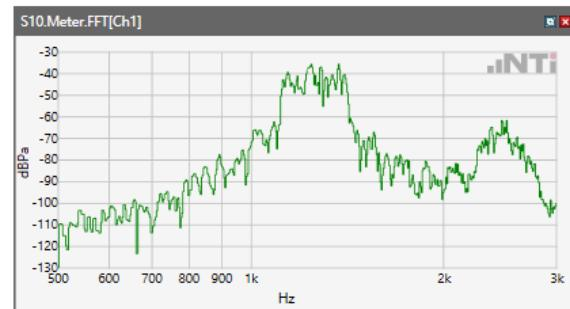
ANSI/TIA 5050-2018 \ 2N HAC ON \ NB 12.2kbps\ 5.2 Receive path – distortion and noise\WCDMA Band II
