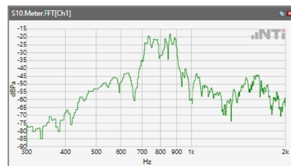
ANSI/TIA 5050-2018 \ 8N HAC OFF \ NB 12.2kbps\ 5.2 Receive path – distortion and noise\LTE Band 5
