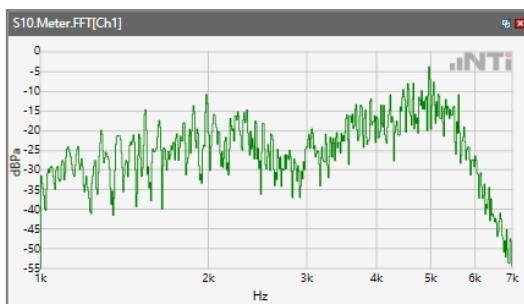
ANSI/TIA 5050-2018 \ 8N HAC OFF \ WB 23.85 kbps\ 5.2 Receive path – distortion and noise\WCDMA II
