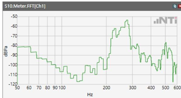
ANSI/TIA 5050-2018 \ 2N HAC ON \ WB 23.85 kbps\ 5.2 Receive path – distortion and noise\ GSM 1900
