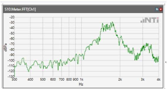
ANSI/TIA 5050-2018 \ 8N HAC OFF \ NB 12.2kbps\ 5.2 Receive path – distortion and noise\WCDMA Band II
