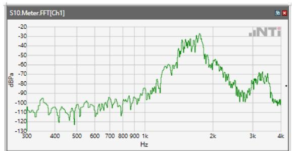
ANSI/TIA 5050-2018 \ 2N HAC ON \ NB 12.2kbps\ 5.2 Receive path – distortion and noise\WCDMA Band II
