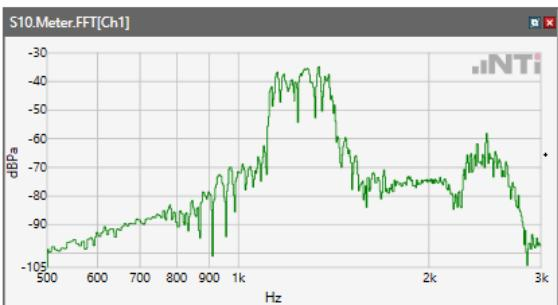
ANSI/TIA 5050-2018 \ 8N HAC OFF \ NB 12.2kbps\ 5.2 Receive path – distortion and noise\WCDMA Band II
