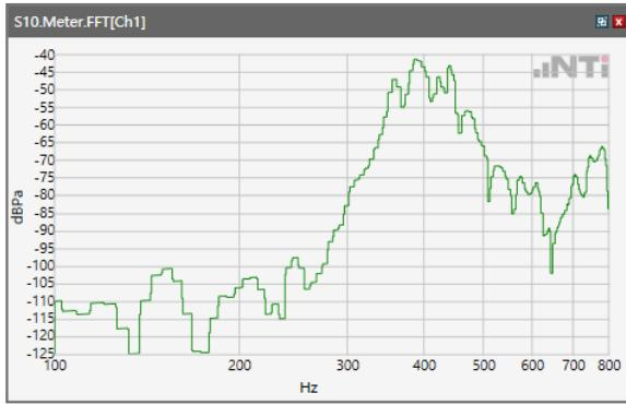
ANSI/TIA 5050-2018 \ 2N HAC ON \ NB 12.2kbps\ 5.2 Receive path – distortion and noise\WCDMA Band II
