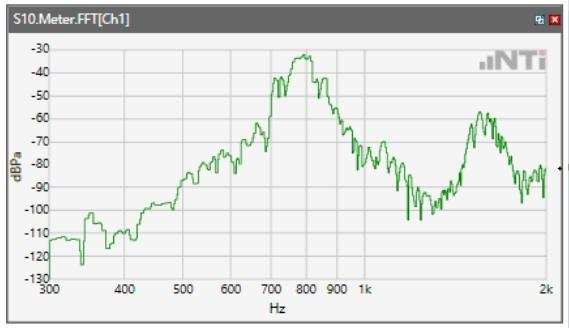
ANSI/TIA 5050-2018 \ 8N HAC OFF \ NB 12.2kbps\ 5.2 Receive path – distortion and noise\GSM 1900
