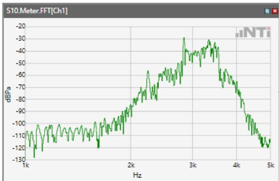
ANSI/TIA 5050-2018 \ 8N HAC OFF \ NB 12.2kbps\ 5.2 Receive path – distortion and noise\ WLAN 2.4GHz
