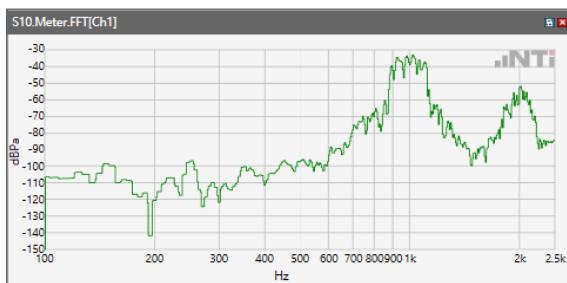
ANSI/TIA 5050-2018 \ 2N HAC ON \ NB 12.2kbps\ 5.2 Receive path – distortion and noise\WCDMA Band IV
