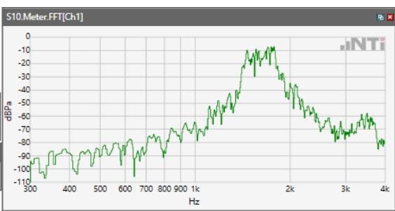
ANSI/TIA 5050-2018 \ 2N HAC ON \ NB 12.2kbps\ 5.2 Receive path – distortion and noise\LTE Band 5
