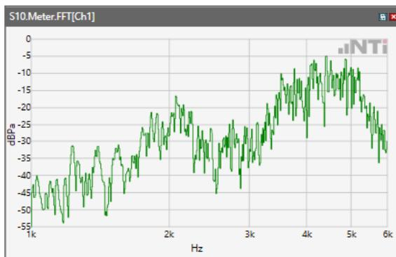
ANSI/TIA 5050-2018 \ 8N HAC OFF \ WB 23.85 kbps\ 5.2 Receive path – distortion and noise\LTE Band 5
