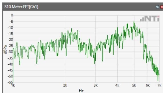
ANSI/TIA 5050-2018 \ 8N HAC OFF \ WB 23.85 kbps\ 5.2 Receive path – distortion and noise\WCDMA V
