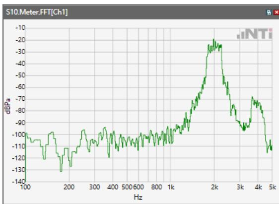
ANSI/TIA 5050-2018 \ 8N HAC OFF \ WB 23.85 kbps\ 5.2 Receive path – distortion and noise\WCDMA IV
