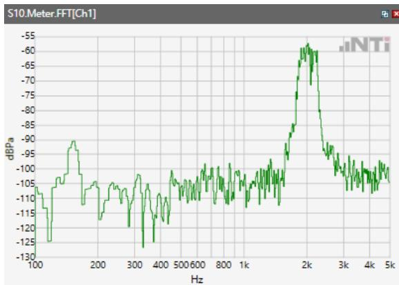
ANSI/TIA 5050-2018 \ 8N HAC OFF \ WB 23.85 kbps\ 5.2 Receive path – distortion and noise\LTE Band 2
