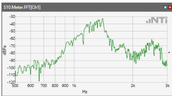
ANSI/TIA 5050-2018 \ 2N HAC ON \ NB 12.2kbps\ 5.2 Receive path – distortion and noise\LTE Band 2
