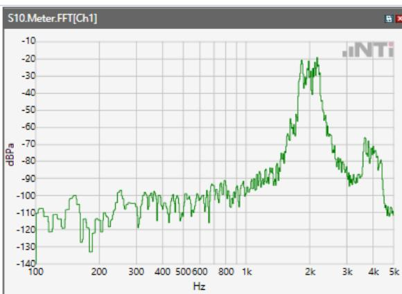
ANSI/TIA 5050-2018 \ 8N HAC OFF \ NB 12.2kbps\ 5.2 Receive path – distortion and noise\WCDMA Band II
