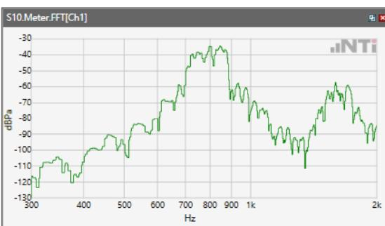
ANSI/TIA 5050-2018 \ 8N HAC OFF \ WB 23.85 kbps\ 5.2 Receive path – distortion and noise\ LTE BAND 71
