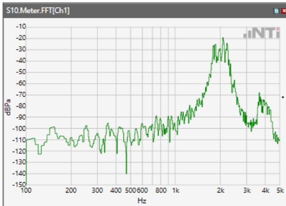
ANSI/TIA 5050-2018 \ 8N HAC OFF \ WB 23.85 kbps\ 5.2 Receive path – distortion and noise\WCDMA II
