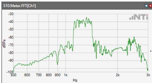
ANSI/TIA 5050-2018 \ 8N HAC OFF \ WB 23.85 kbps\ 5.2 Receive path – distortion and noise\WCDMA V
