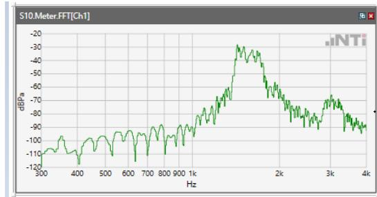
ANSI/TIA 5050-2018 \ 8N HAC OFF \ WB 23.85 kbps\ 5.2 Receive path – distortion and noise\WCDMA V
