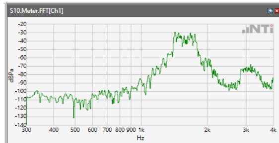
ANSI/TIA 5050-2018 \ 8N HAC OFF \ WB 23.85 kbps\ 5.2 Receive path – distortion and noise\WCDMA II
