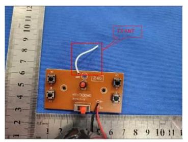
Length: 40mm Antenna Type: Wire Antenna Antenna Gain: 0dBi
