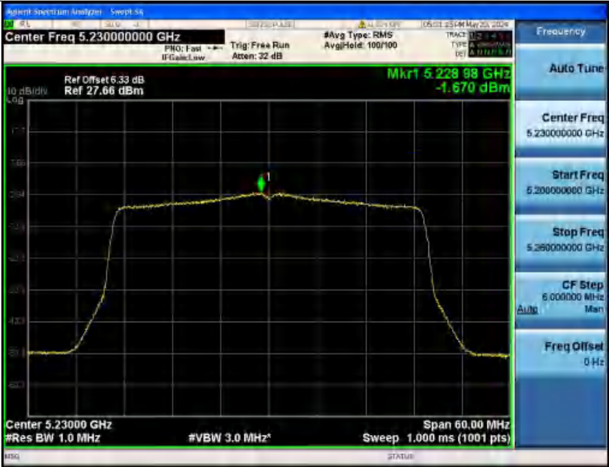
Power Spectral Density NVHT_ANT2 802_11ax(HE40) 5230
