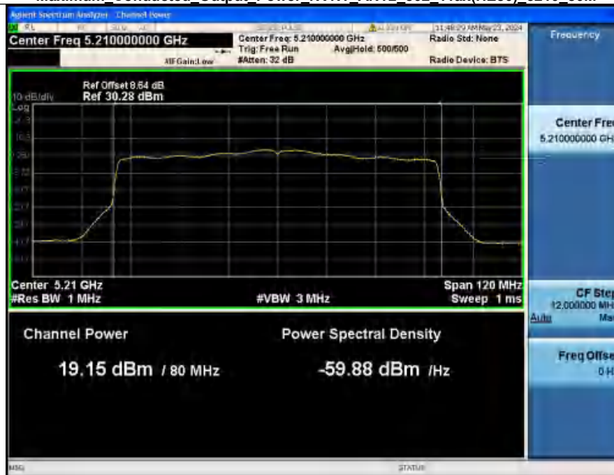
Maximum Conducted Output Power NVNT ANT2_802_11ax(HE80) 5210 80M
