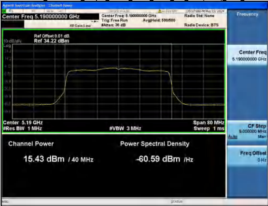
Maximum Conducted Output Power NVHT ANT2_802_11ax(HE40) 5190_40M
