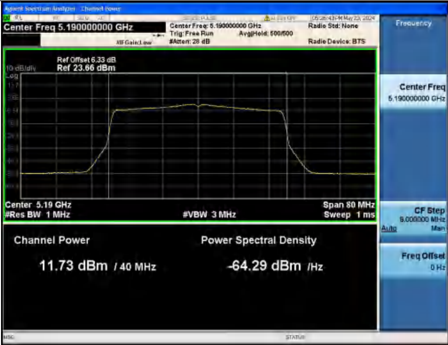
Maximum Conducted Output Power NVHT ANT2_802_11ax(HE40) 5190_40M
