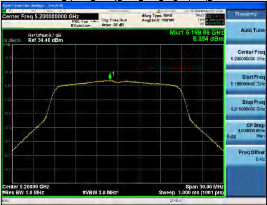
Power Spectral Density NVNT ANT2_802_11n(HT20)_5200
