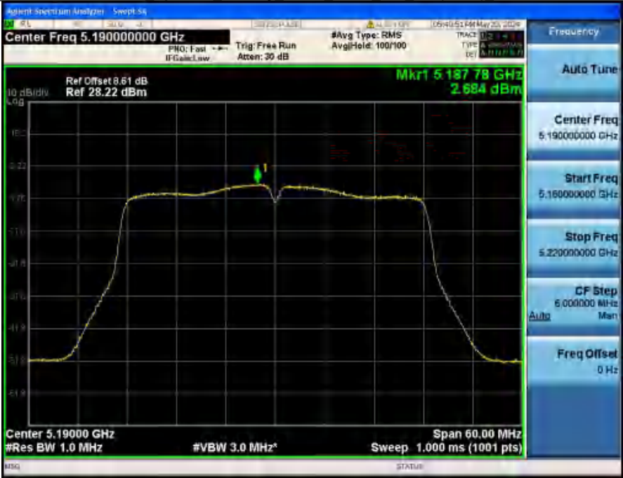
Power Spectral Density NVHT ANT2_802_11n(HT40)_5190
