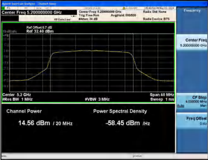
Maximum Conducted Output Power NVHT ANT2_802_11ax(HE20)_5200_20M
