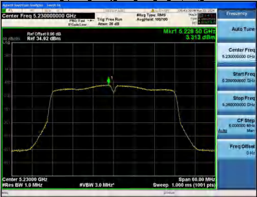
Power Spectral Density NVHT ANT2_802_11n(HT40)_5230
