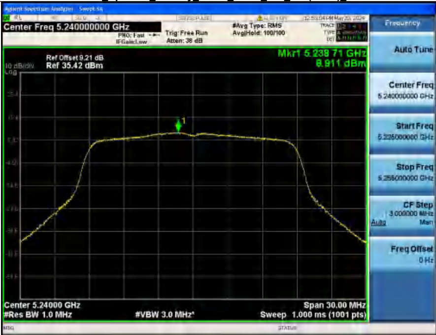
Power Spectral Density NVNT ANT2_802_11n(HT20)_5240
