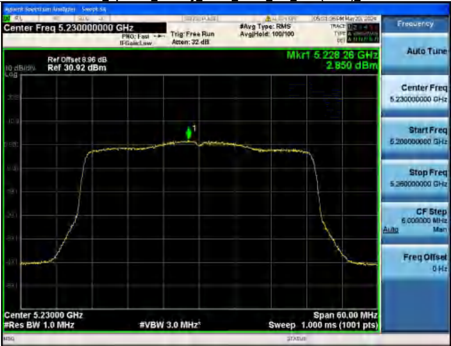
Power Spectral Density NVHT_ANT2 802_11ax(HE40) 5230
