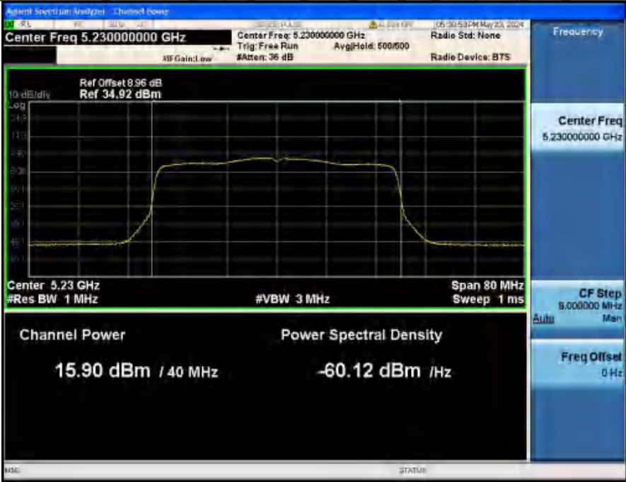
Maximum Conducted Output Power NVHT ANT2_802_11ax(HE40)_5230_40M
