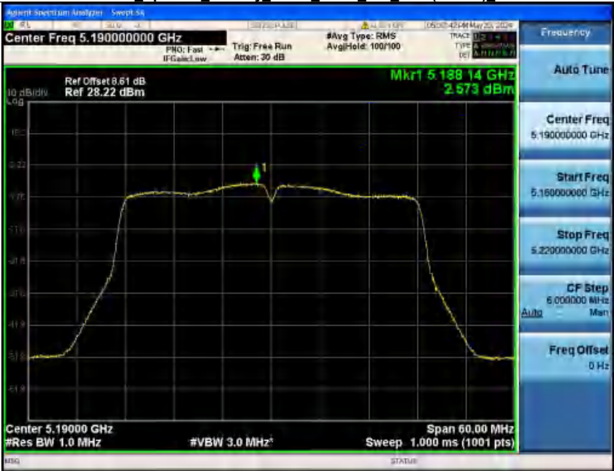
Power Spectral Density NVHT_ANT2_802_11ac(VHT40)_5190
