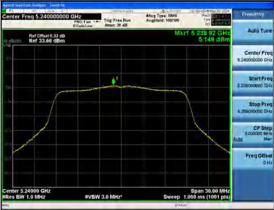
Power Spectral Density NVNT ANT2_802_11n(HT20)_5240
