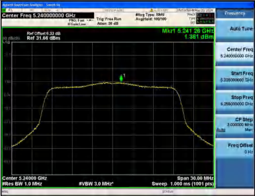
Power Spectral Density NVHT_ANT2_802_11ax(HE20)_5240
