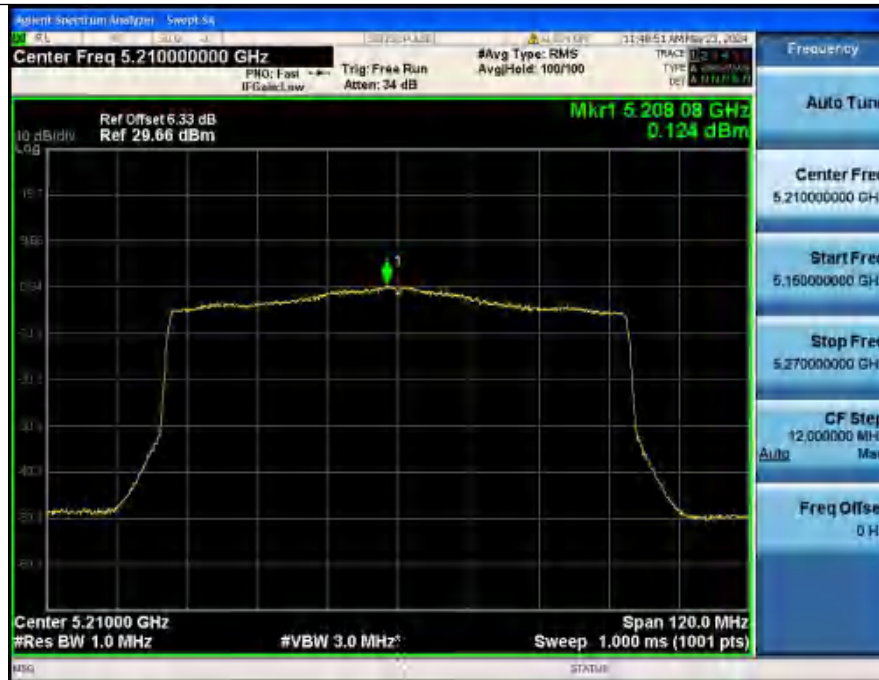
Power Spectral Density NVNT ANT2 802.11ax(HE80) 5210
