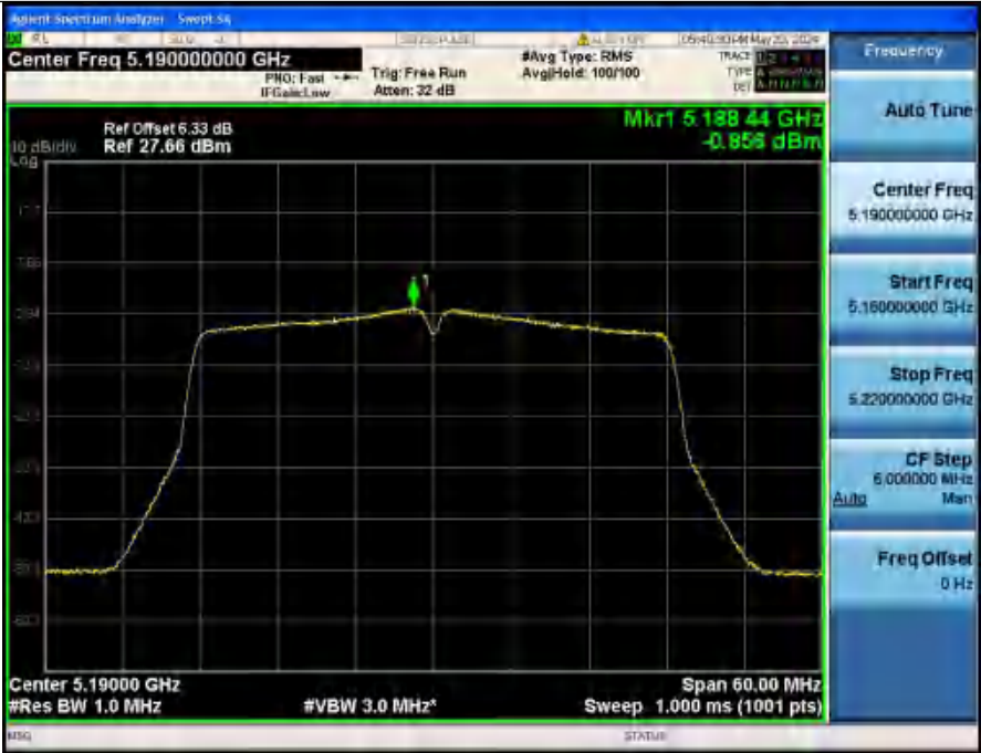
Power Spectral Density NVHT ANT2_802_11n(HT40)_5190
