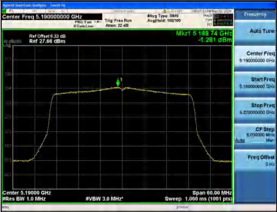
Power Spectral Density NVHT_ANT2_802_11ax(HE40)_5190
