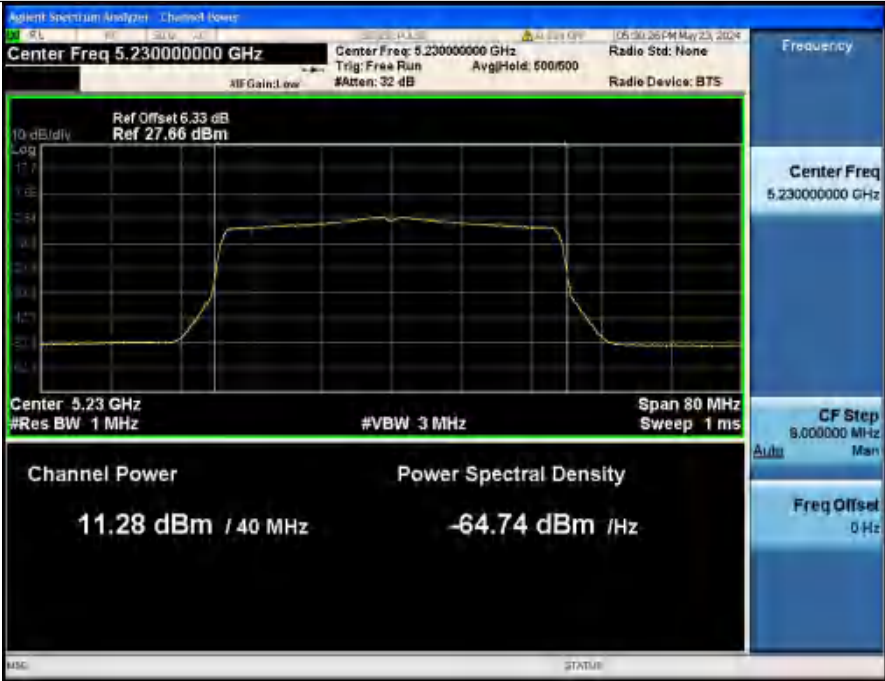
Maximum Conducted Output Power NVHT ANT2_802_11ax(HE40)_5230_40M
