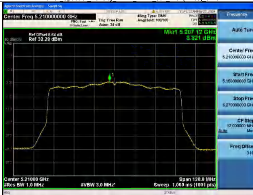
Power Spectral Density NVNT ANT2 802.11ax(HE80) 5210
