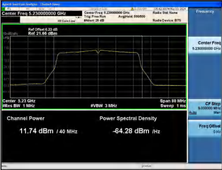
Maximum_Conducted_Output_Power_NVHT_ANT2_802_11n(HT40)_5230_40M
