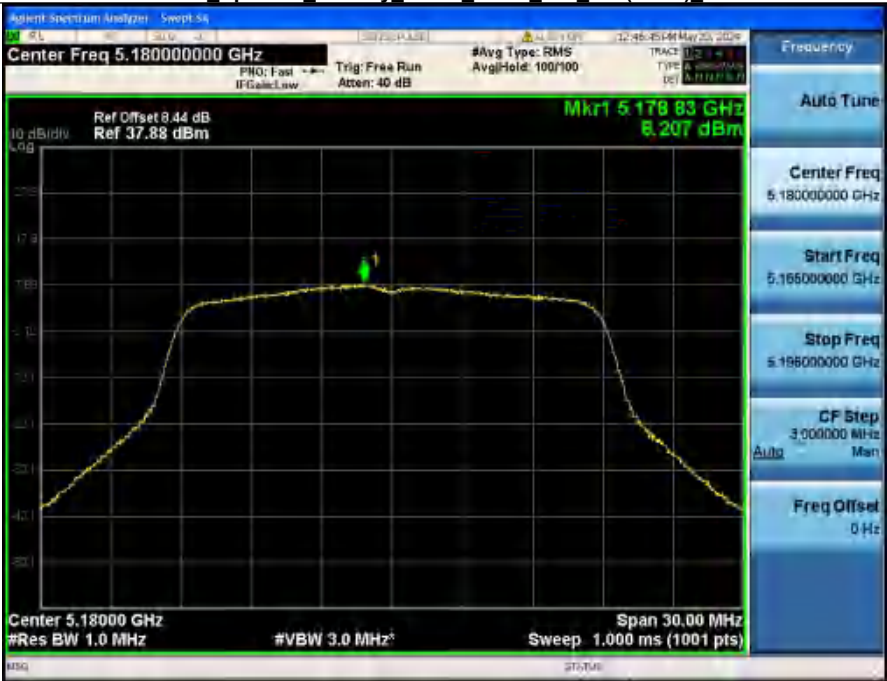
Power Spectral Density NVNT ANT2_802_11n(HT20)_5180
