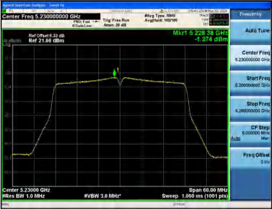
Power Spectral Density NVHT ANT2_802_11n(HT40)_5230
