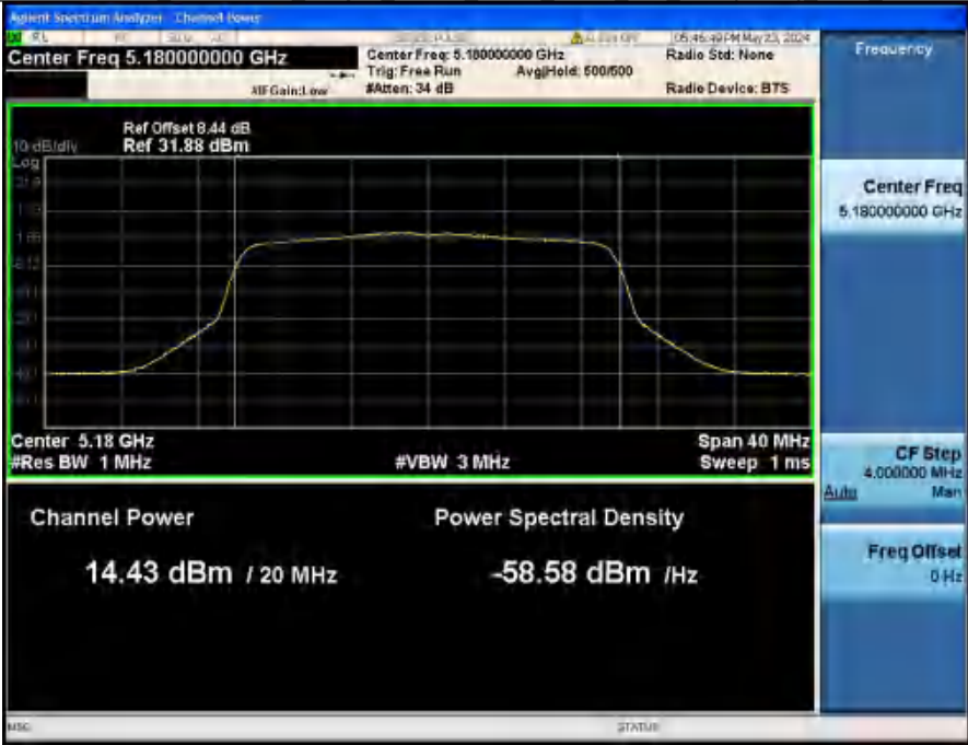
Maximum Conducted Output Power NVHT_ANT2_802_11ax(HE20)_5180_20M
