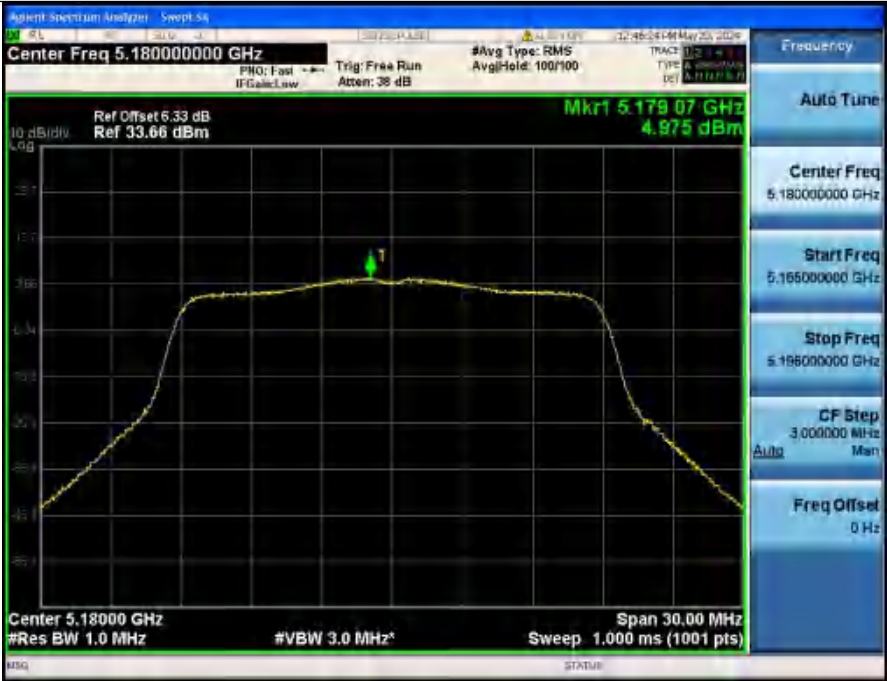
Power Spectral Density NVNT ANT2_802_11n(HT20)_5180
