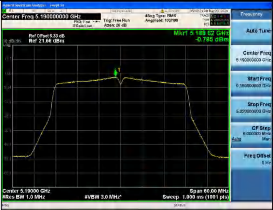
Power Spectral Density NVHT_ANT2_802_11ac(VHT40)_5190
