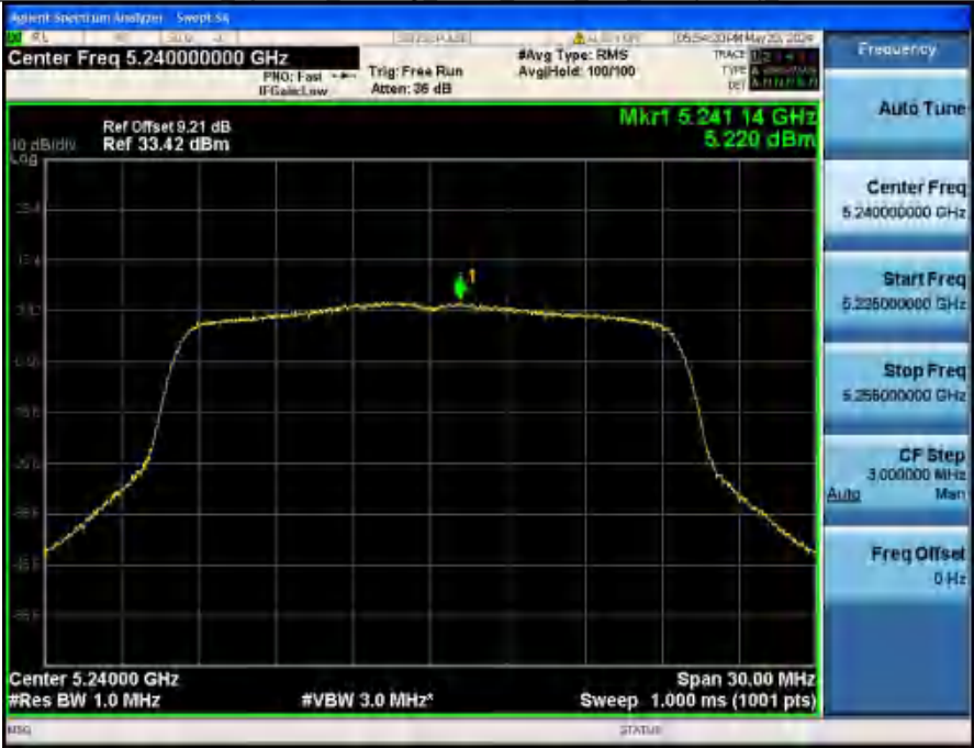
Power Spectral Density NVHT_ANT2_802_11ax(HE20)_5240
