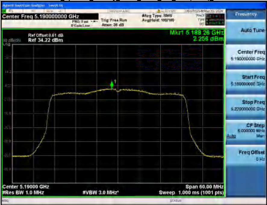
Power Spectral Density NVHT_ANT2_802_11ax(HE40)_5190
