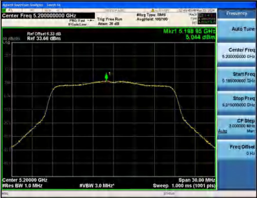
Power Spectral Density NVNT ANT2_802_11n(HT20)_5200
