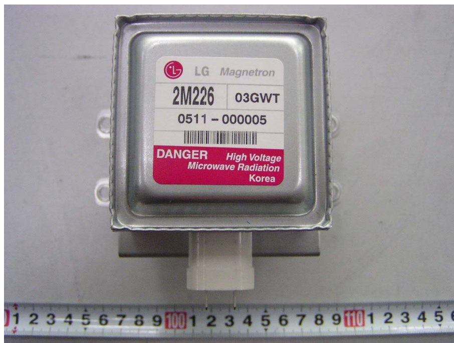
EUT-Magnetron Top View
