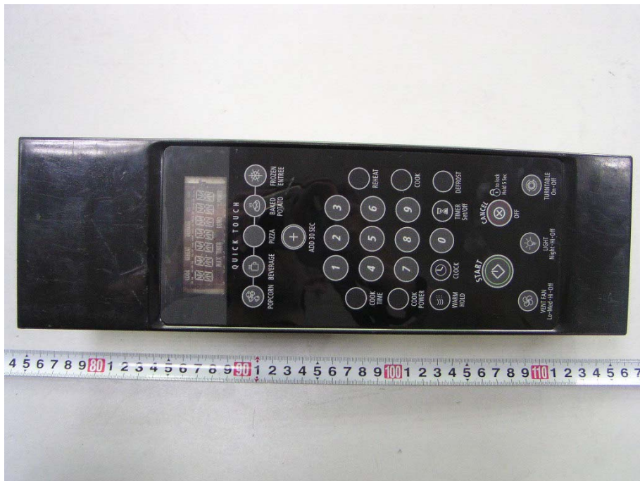
EUT-Control Unit Top View
