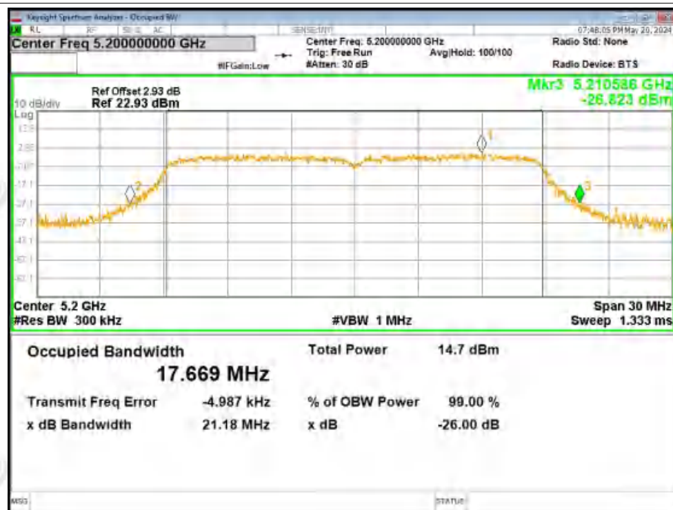
-26dB Bandwidth NVNT ac20 5240MHz Ant2
