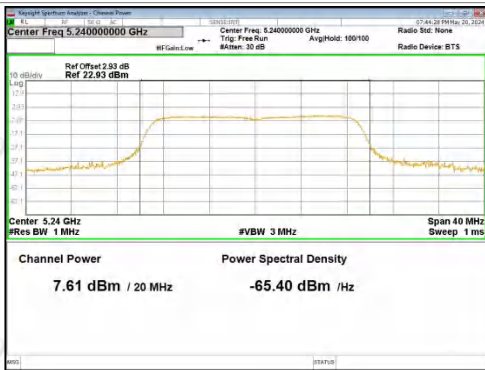
Power NVNT n20 5240MHz Ant2
