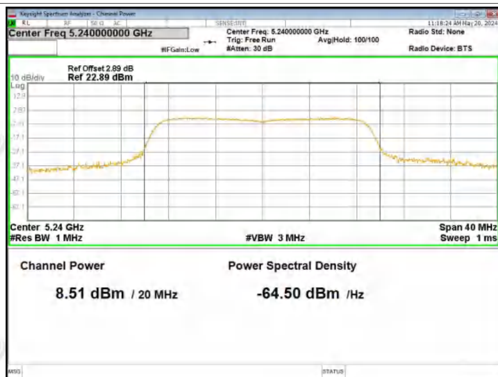
Power NVNT n20 5180MHz Ant2
