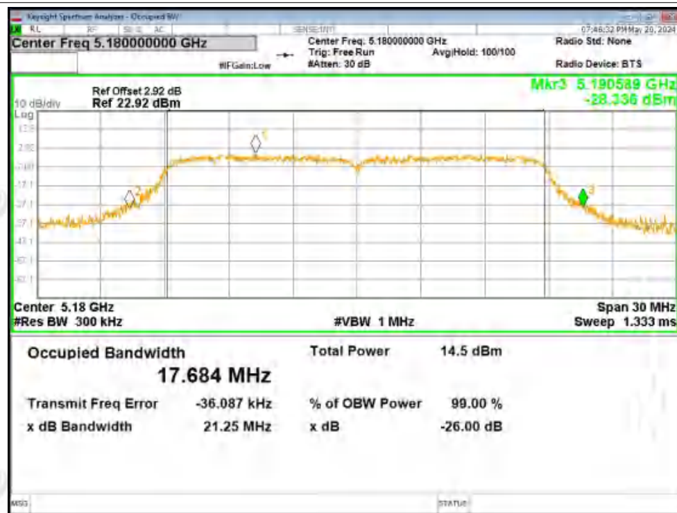
-26dB Bandwidth NVNT ac20 5180MHz Ant2
