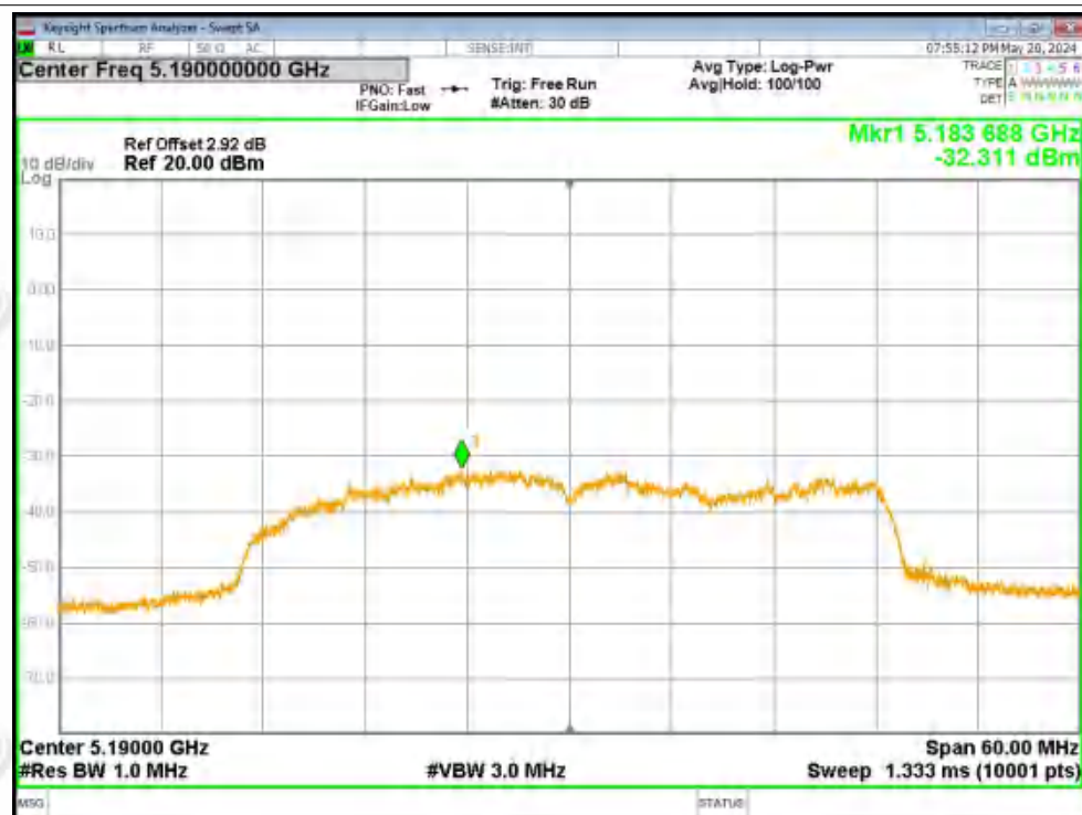
PSD NVNT ac40 5230MHz Ant2
