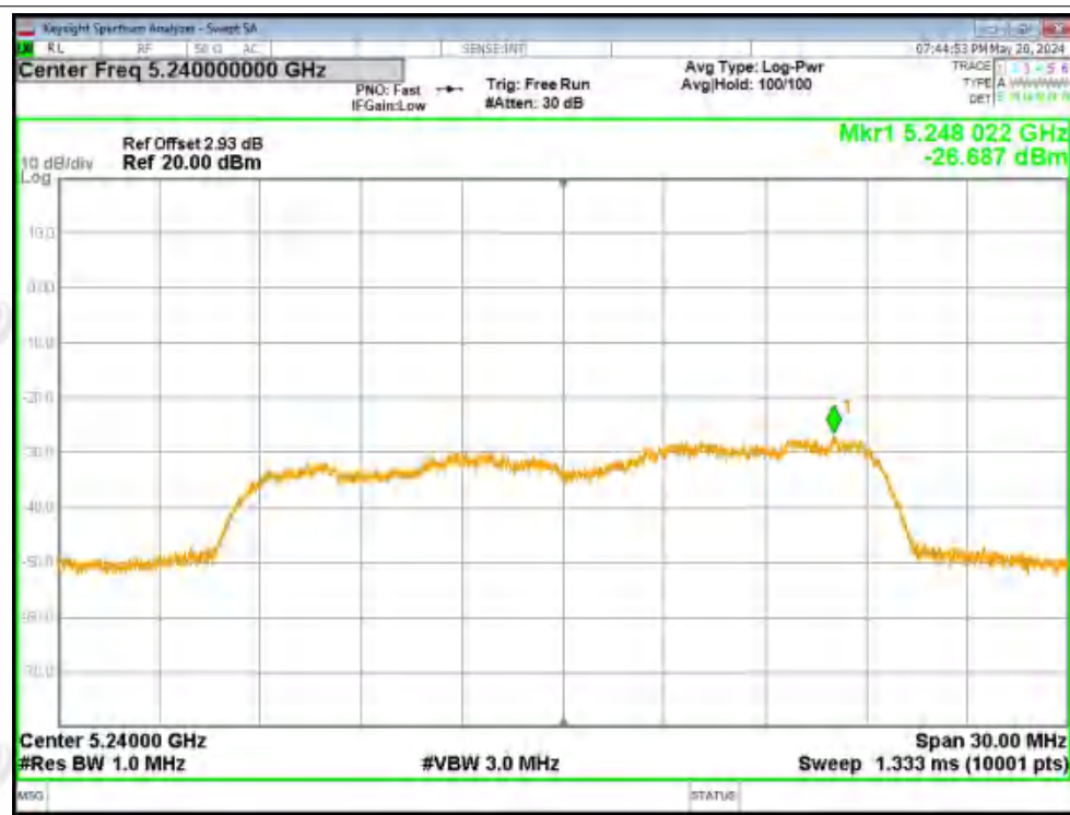
PSD NVNT n20 5240MHz Ant2
