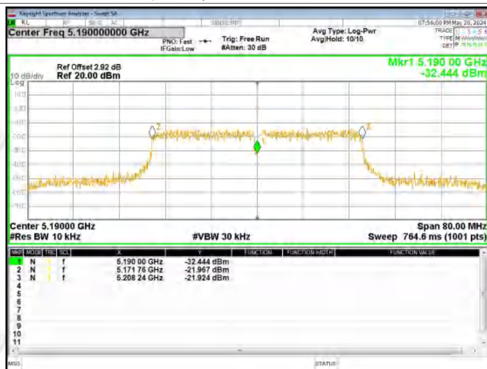
Freq. Stability NVNT ac40 5230MHz Ant2
