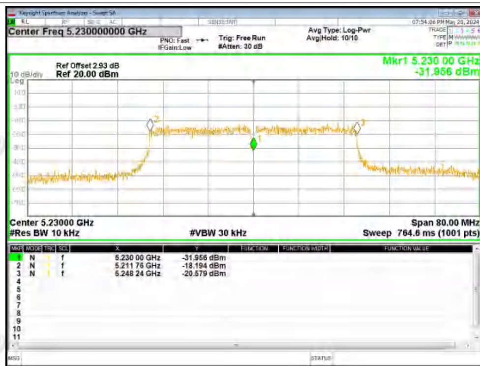
Freq. Stability NVNT n40 5230MHz Ant2
