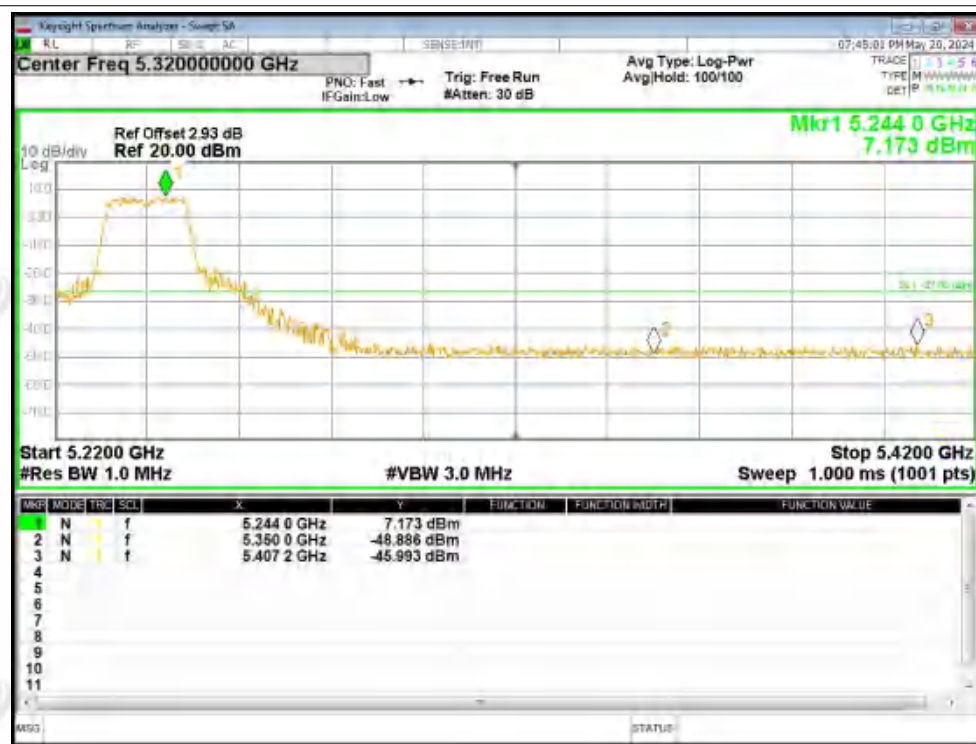
Band Edge NVNT n20 5240MHz High Ant2
