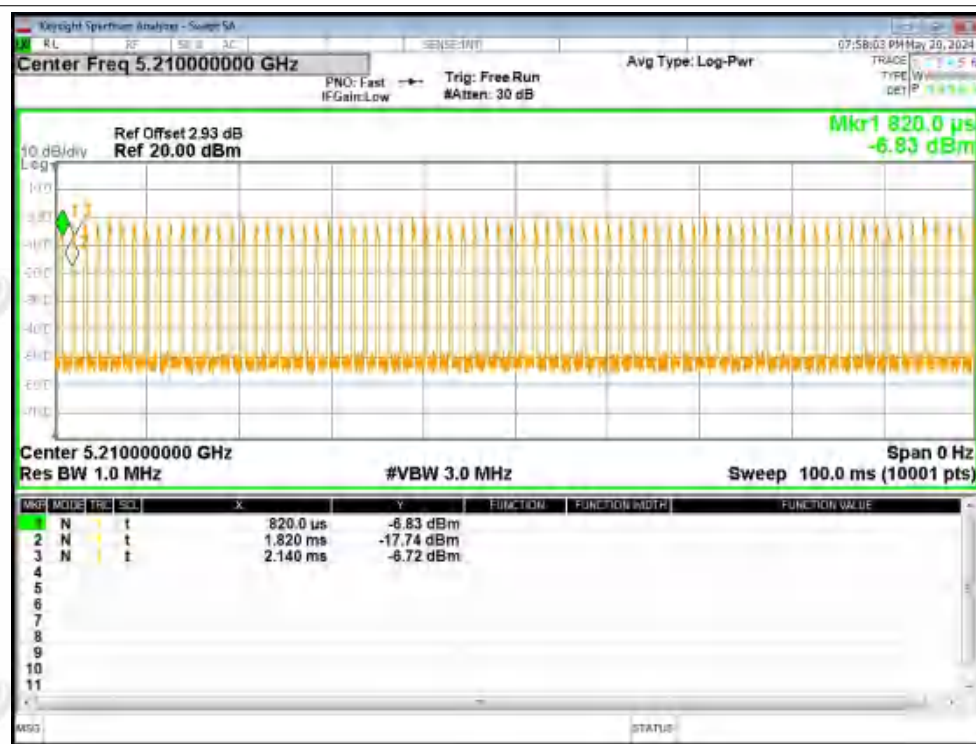
Duty Cycle NVNT ac80 5210MHz Ant2
