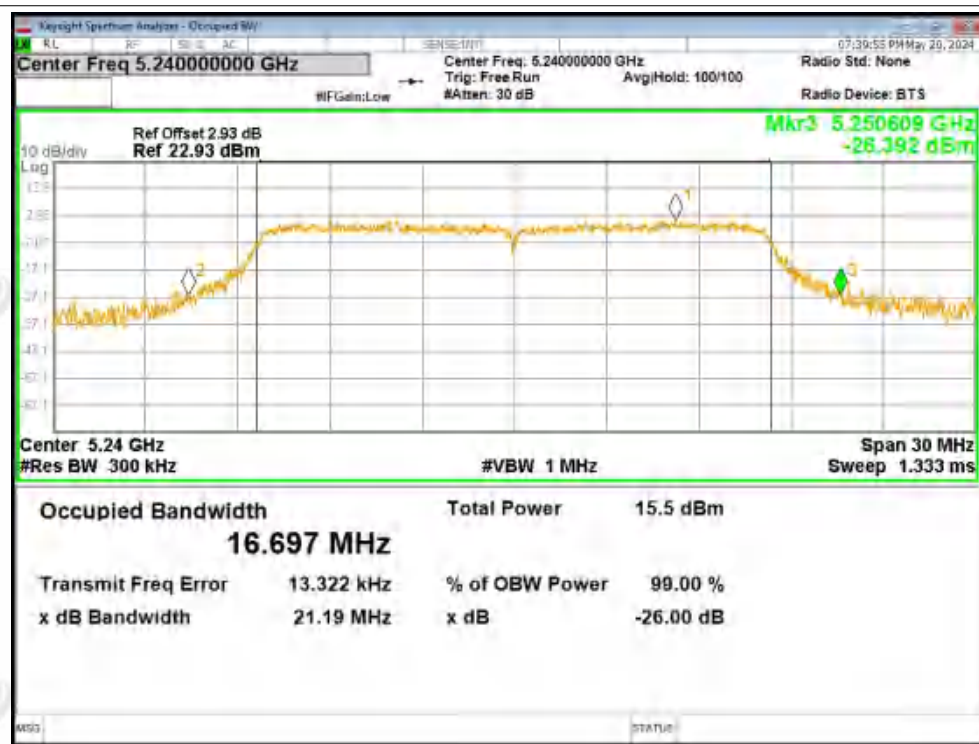
-26dB Bandwidth NVNT a 5240MHz Ant2
