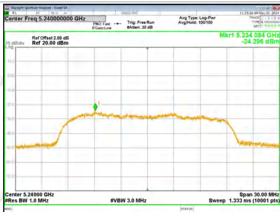
PSD NVNT ac20 5180MHz Ant2
