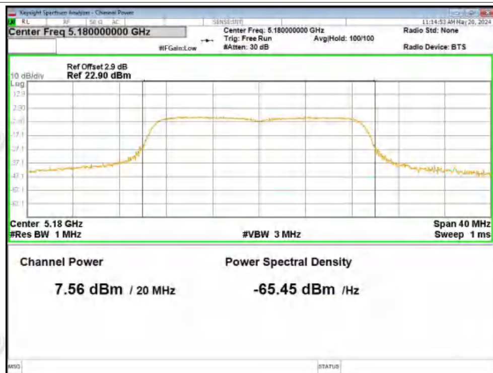
Power NVNT n20 5200MHz Ant1
