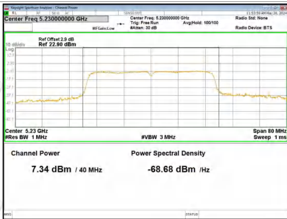
Power NVNT ac40 5230MHz Ant1
