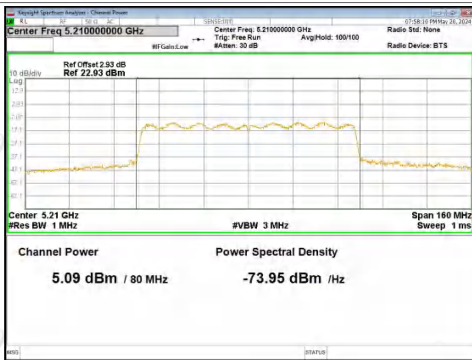
Power NVNT ac80 5210MHz Ant2
