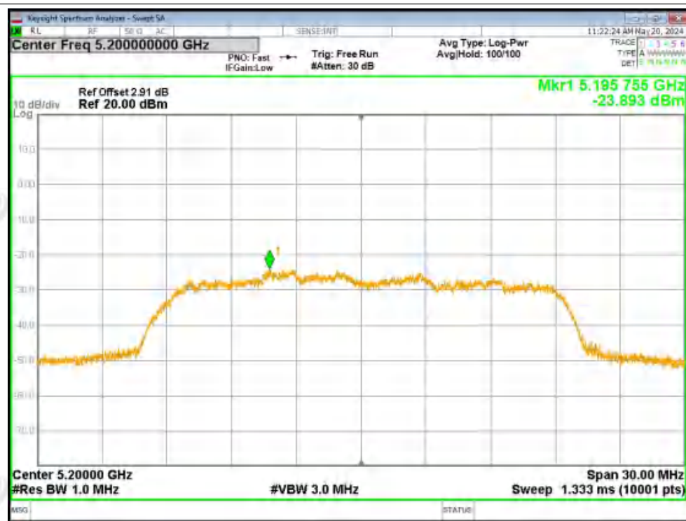
PSD NVNT ac20 5200MHz Ant1
