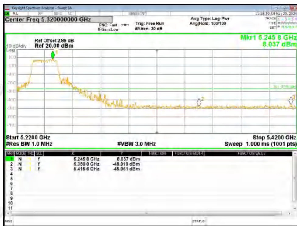
Band Edge NVNT n20 5240MHz High Ant1
