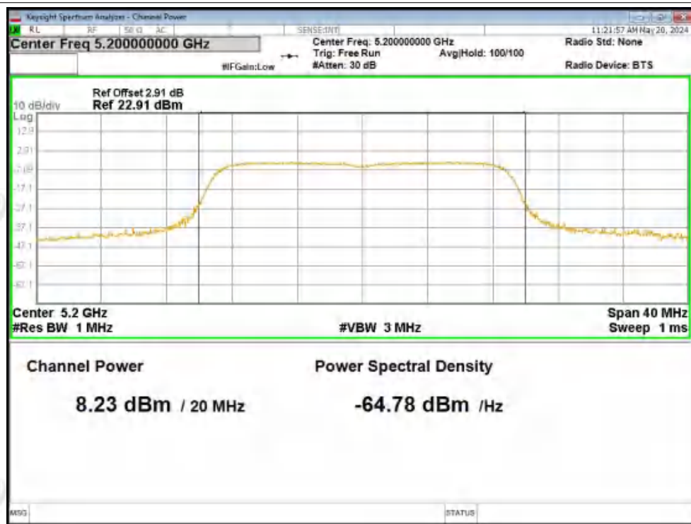
Power NVNT ac20 5200MHz Ant1
