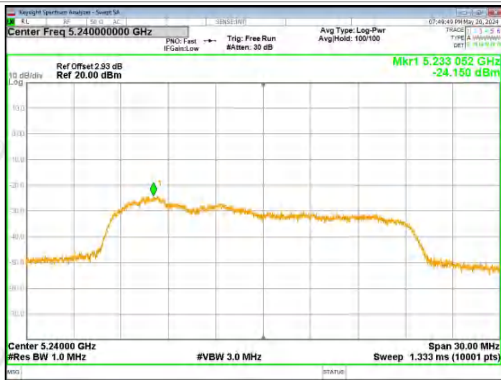
PSD NVNT ac20 5240MHz Ant2
