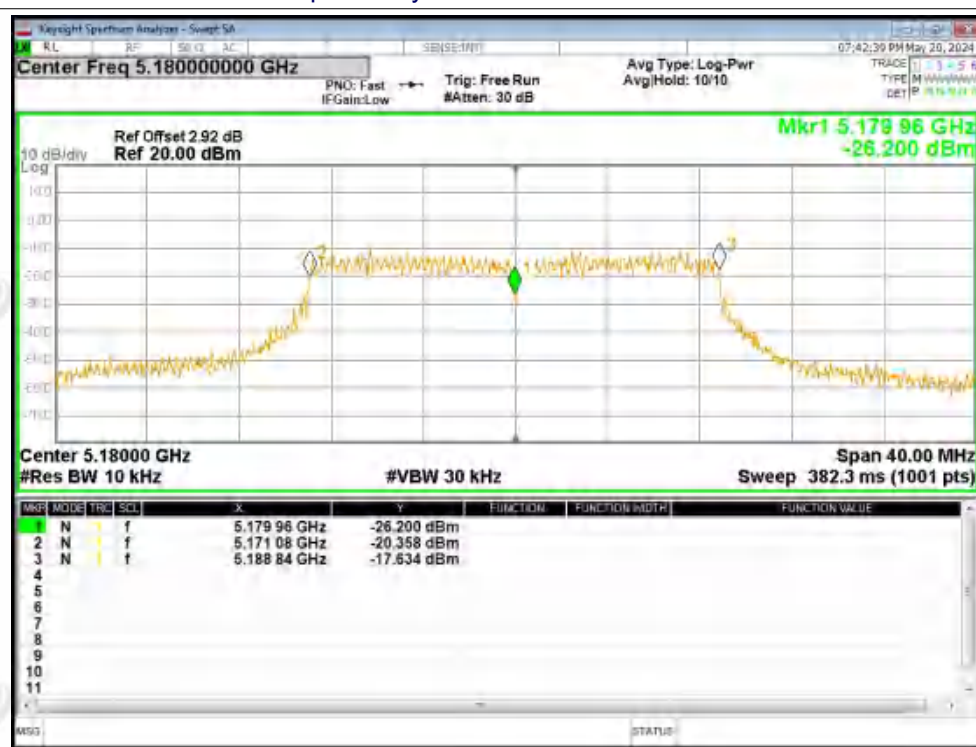
Freq. Stability NVNT n20 5180MHz Ant2
