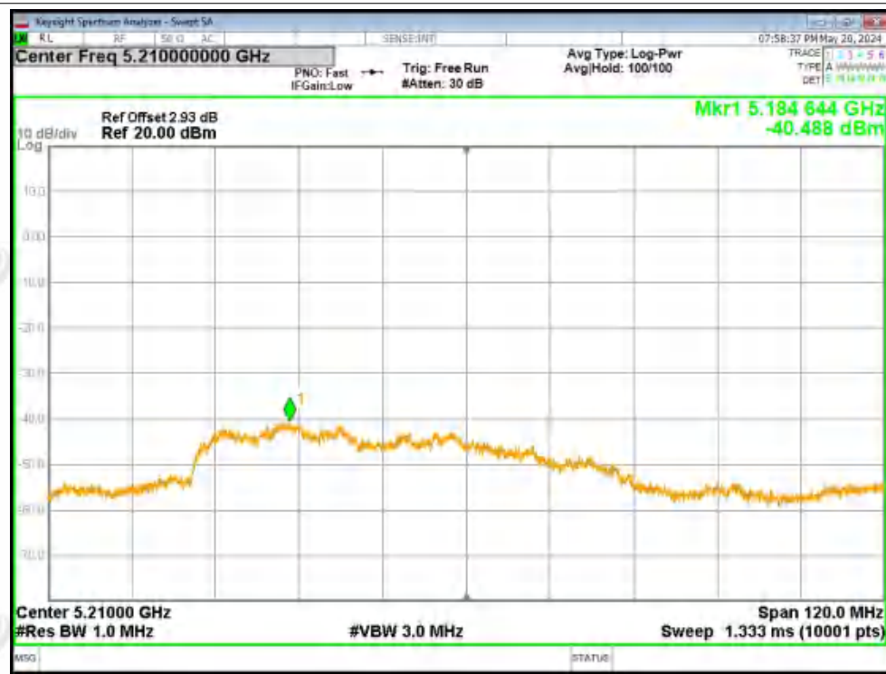
PSD NVNT ac80 5210MHz Ant2
