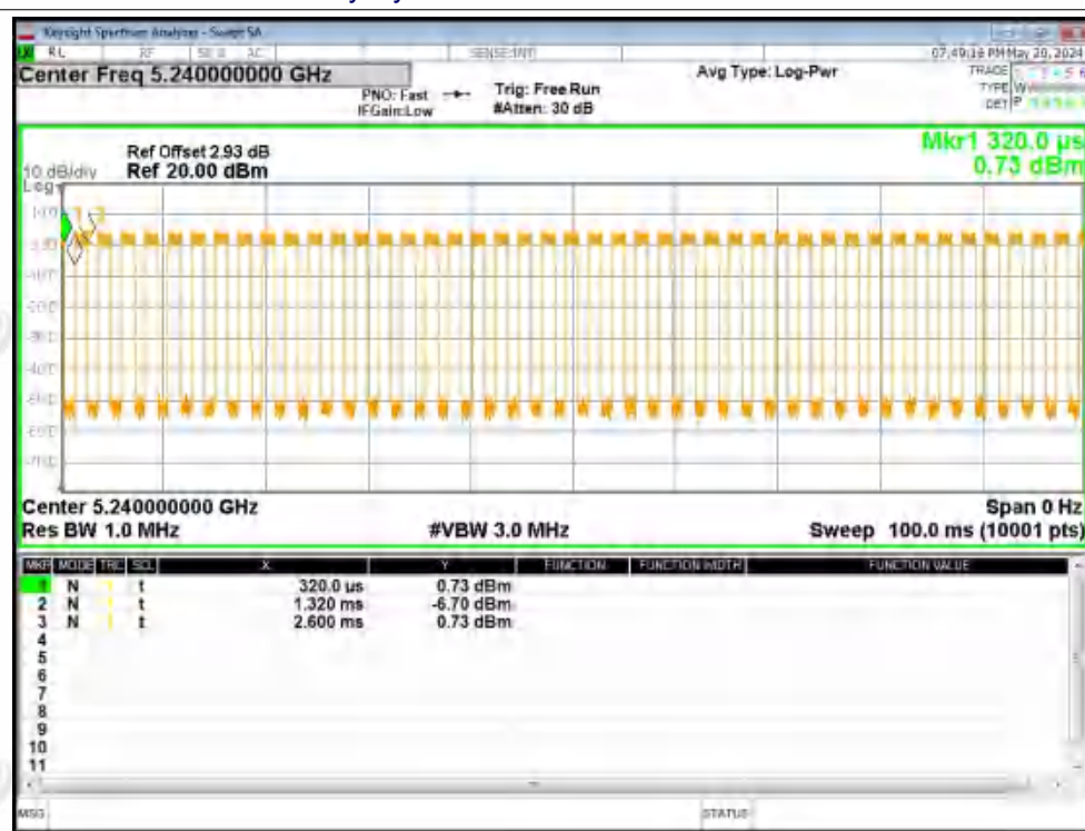
Duty Cycle NVNT ac20 5240MHz Ant2
