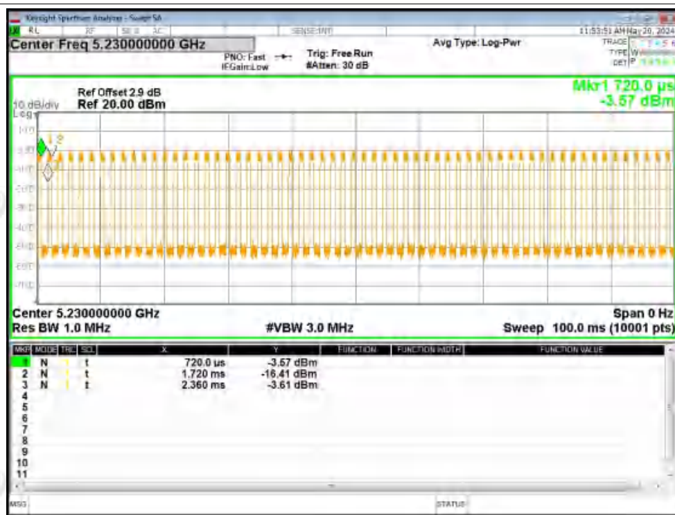
Duty Cycle NVNT ac40 5230MHz Ant1
