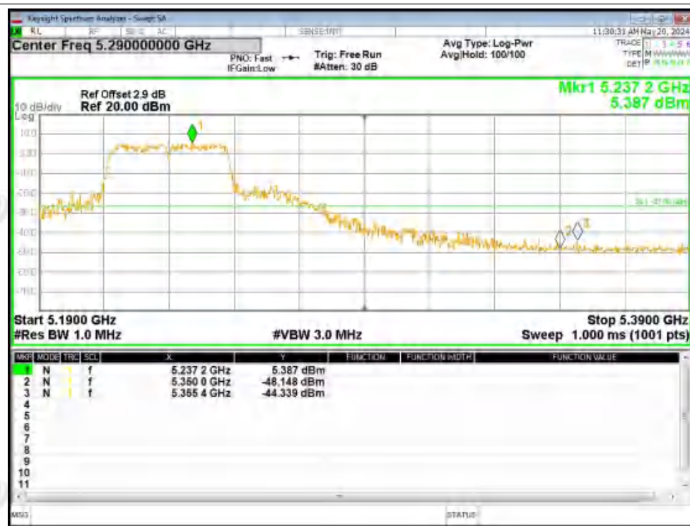
Band Edge NVNT n40 5230MHz High Ant1
