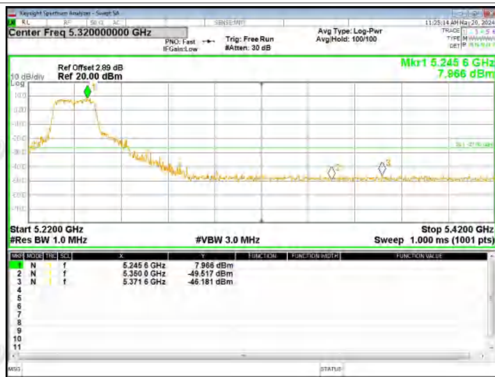
Band Edge NVNT ac20 5240MHz High Ant1
