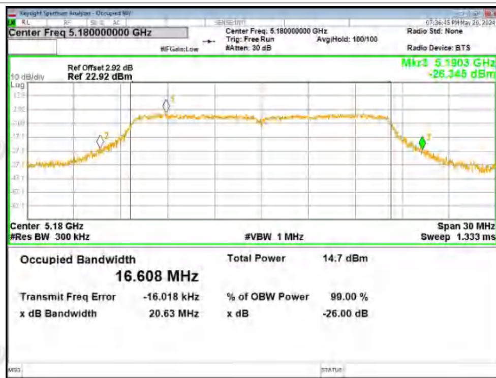
-26dB Bandwidth NVNT a 5180MHz Ant2
