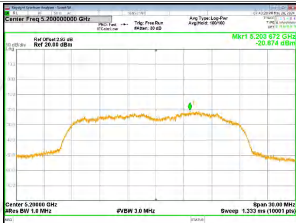
PSD NVNT n20 5240MHz Ant2
