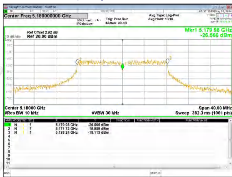
Freq. Stability NVNT a 5180MHz Ant2
