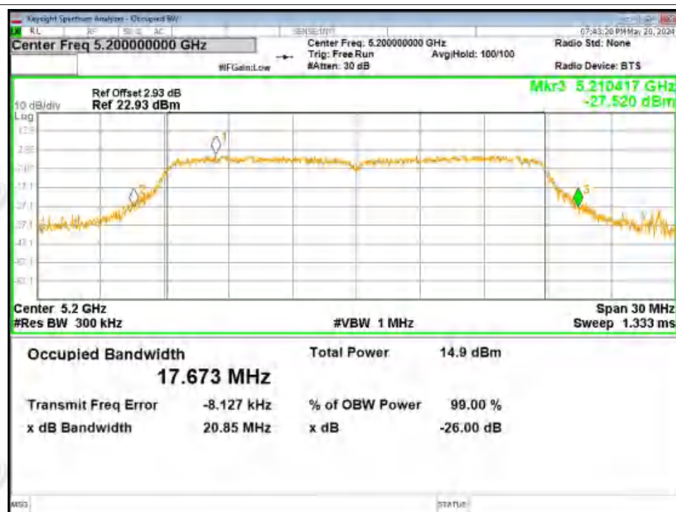
-26dB Bandwidth NVNT n20 5240MHz Ant2
