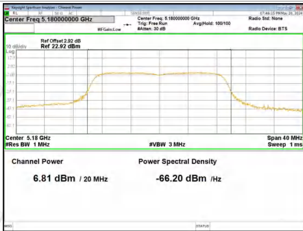
Power NVNT ac20 5180MHz Ant2
