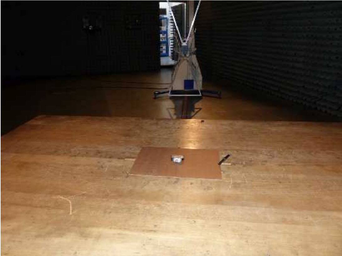
Photo 3, 4, 5: Test setup for radiated measurements, EUT in vertical position Enclosure, semi-anechoic chamber, 30 MHz to 1 GHz, intentional radiator §15
