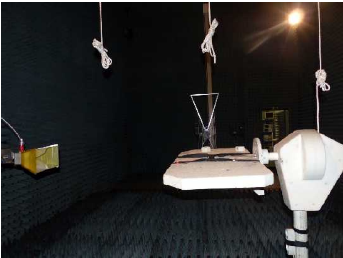
Photo 6, 7: Test setup for radiated measurements, EUT in horizontal position Enclosure, fully-equipped anechoic chamber, 1-4,5 GHz §15
