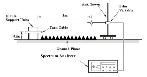
The radiated emission tests were performed in the 3 meters test site.
