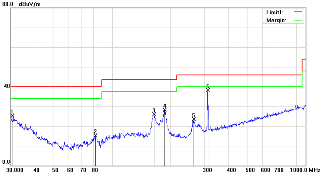
Horizontal Polarity Plot @3m
