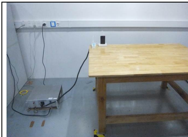
Conducted Emissions Test Setup Front View
