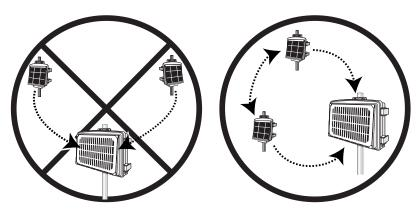
• Nodes can also be used to transmit data around or over obstacles, such as hills.
