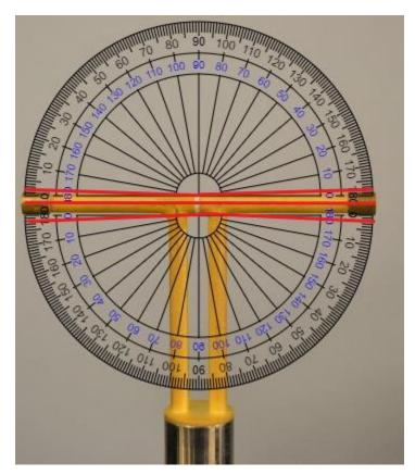
$\bullet~$  The center red line indicates that the arms of the dipole fall within  $\pm 2^{\circ}$
