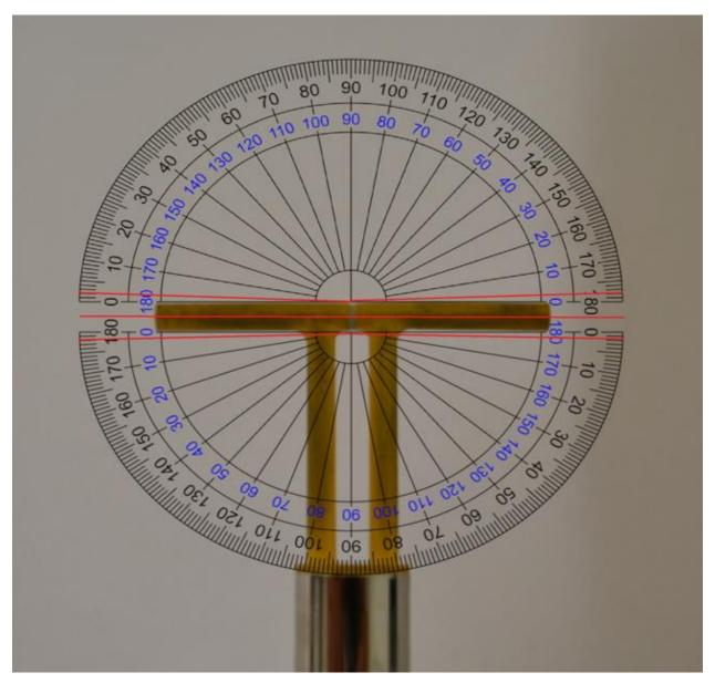
• The center red line indicates that the arms of the dipole fall within  $\pm 2^\circ$
