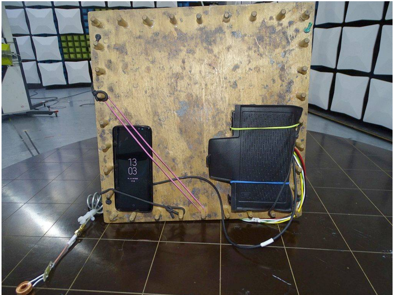
Photo 7: Test setup for radiated measurements (Enclosure, semi-anechoic chamber, NFC external antenna, detail)
