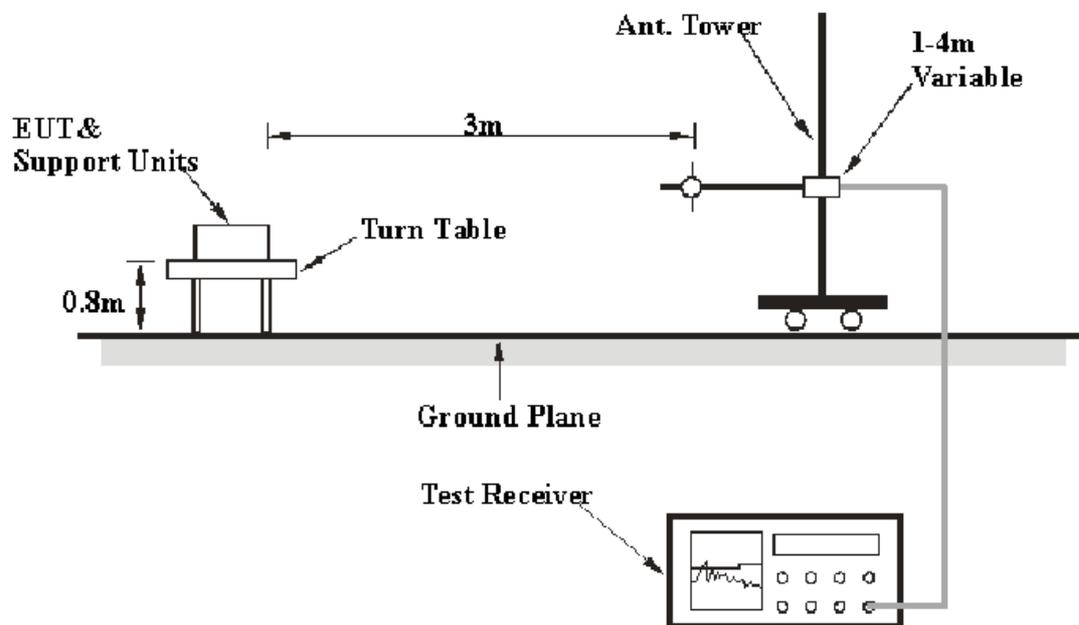
The radiated emission tests were performed in the 3-meter Chamber B, using the setup accordance with the ANSI C63.4-2003. The specification used was the FCC 15.209 and FCC 15.249 limits.
