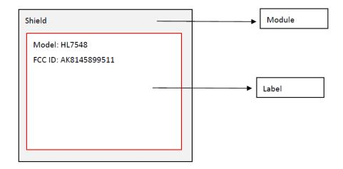
FCC ID is described on top of Module. Labeling meets the conditions allowed in KDB784748. FCC part15 statement in manual, when it would be embeded on Host.
