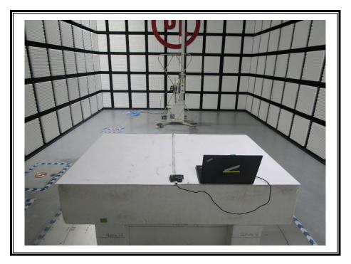
RADIATED RF MEASUREMENT SETUP (30MHz~1GHz) (Y axis)
