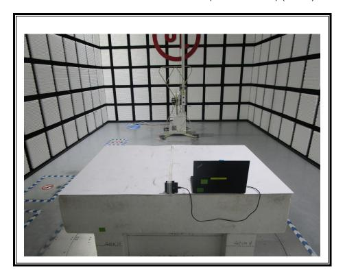
RADIATED RF MEASUREMENT SETUP (Below 30MHz)
