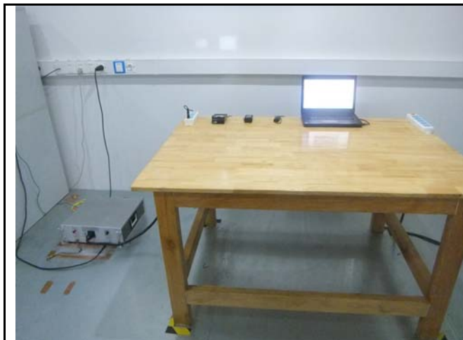
Conducted Emissions Test Setup Front View
