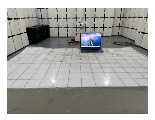
Set-up for Radiated Spurious Emission, Above 1GHz
